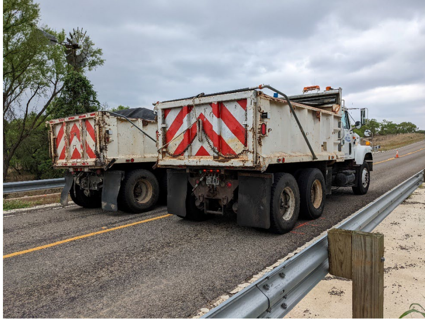
Figure 2-2: Two loading trucks on Bridge 05
