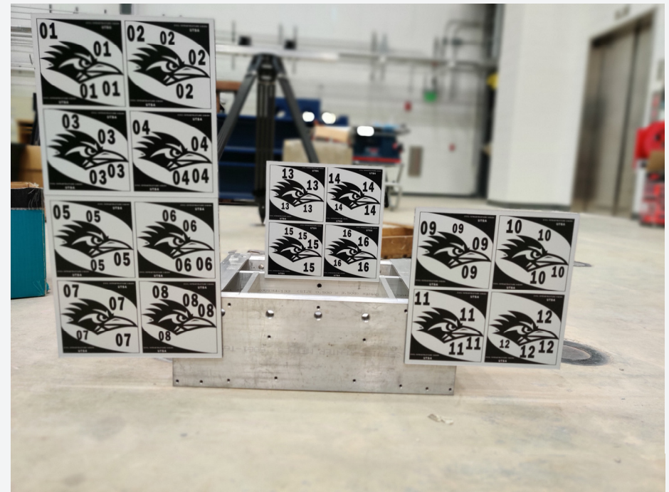
Gage Block Test device setup for acquiring translation data in Z-direction
