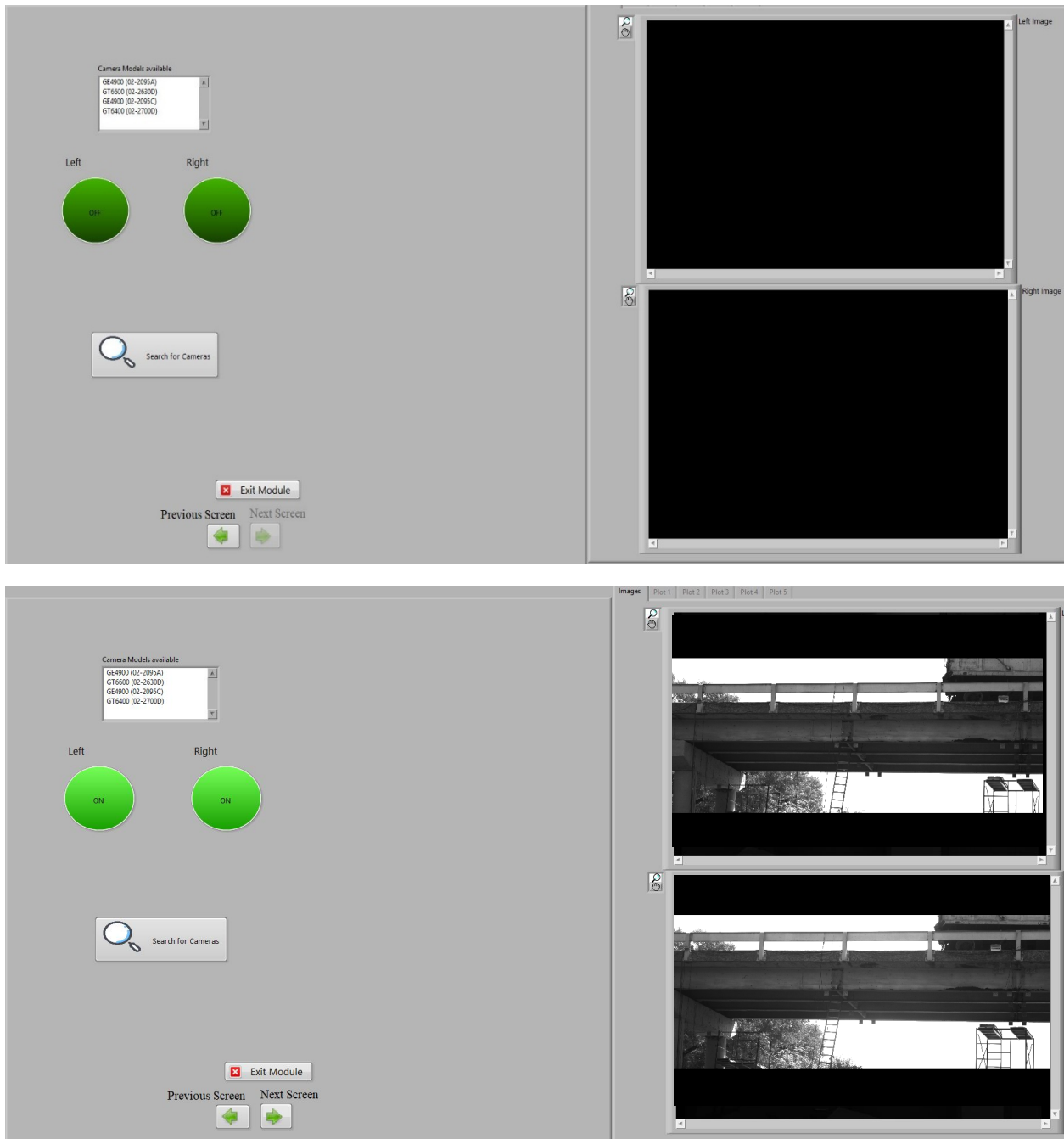
Figure 4-7: Camera Detection screen showing dark green markers (top) when the cameras are not detected and light green (bottom) when they are detected.
