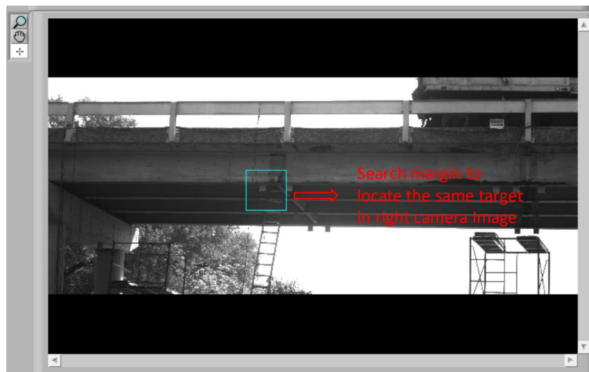
Figure 4-15: Moving the search window to locate the same target in the Right camera image
