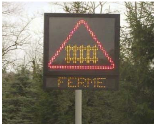
Figure 2-3 VMS in Protected Crossing (Ref. 24)
