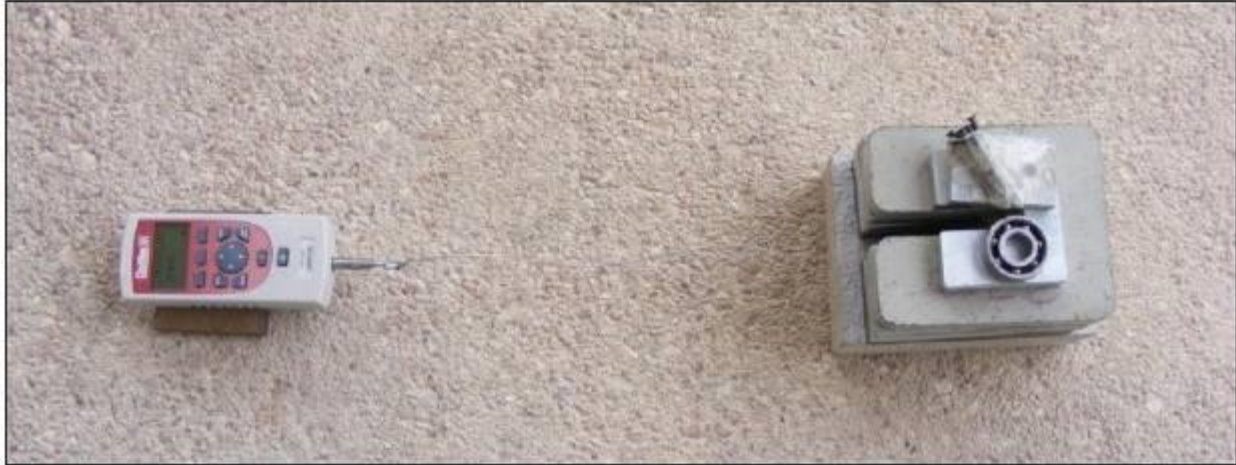
Figure 4.1. Horizontal Dynamometer Pull Meter and a Heel Assembly.
