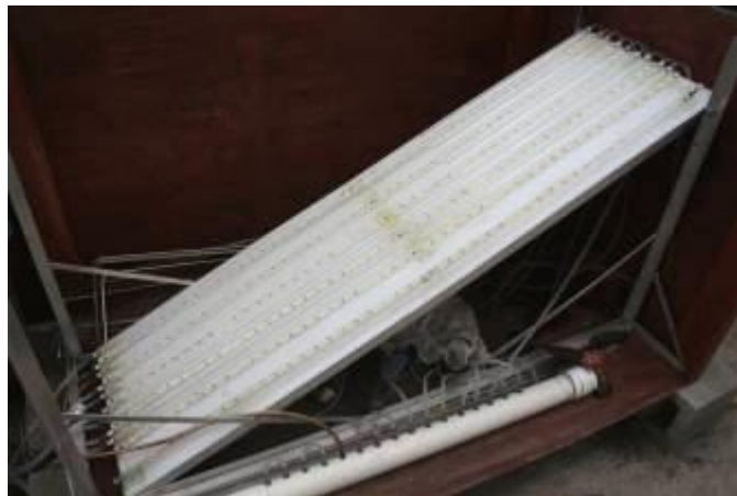
Figure 3.16. Inclined Manometer Board.
