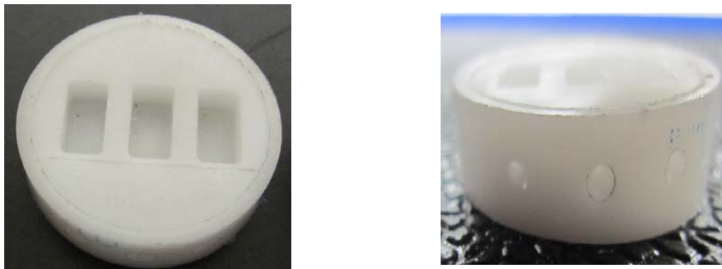
Figure 5.3 – Views of a Finished Delrin Electrode Holder.
