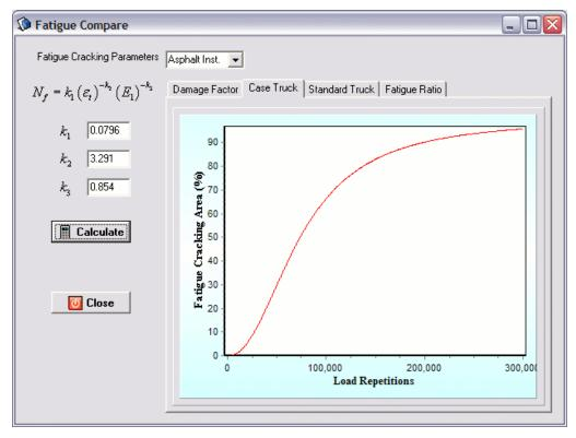
Figure 27 – Fatigue cracking based on load repetitions results per truck.
