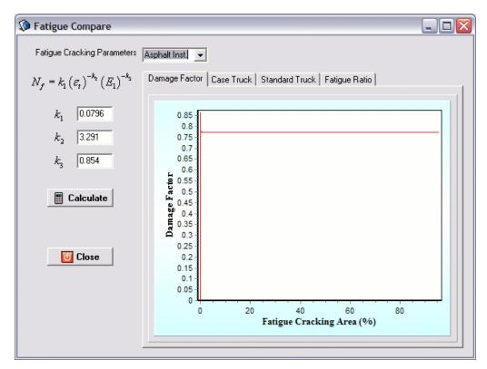
Figure 26 – Damage ratio based on fatigue cracking.
