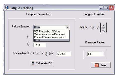
Figure 36 – Available fatigue equations.
