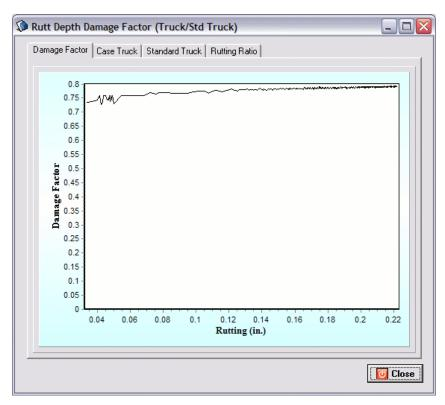
Figure 23 – Damage ratio based on rutting.
