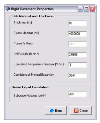
Figure 28 – Rigid pavement properties.
