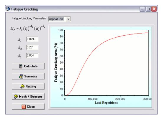
Figure 14 – Fatigue cracking results.
