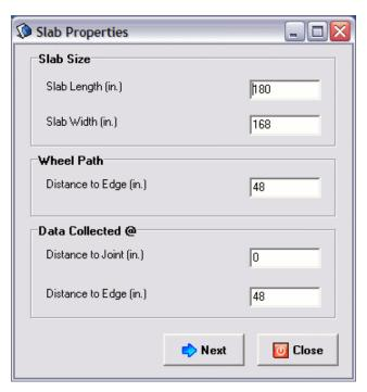
Figure 29 – Rigid pavement properties.
