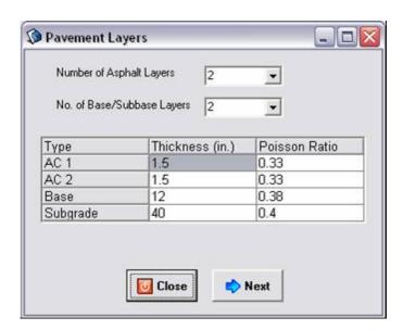
Figure 5 – Number of pavement layers and structural properties.
