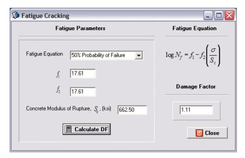
Figure 35 – Damage factor based on fatigue cracking at user defined point.
