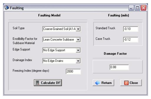
Figure 39 – Faulting model.
