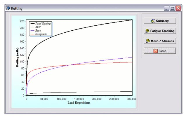
Figure 13 – Rutting vs. load repetitions.
