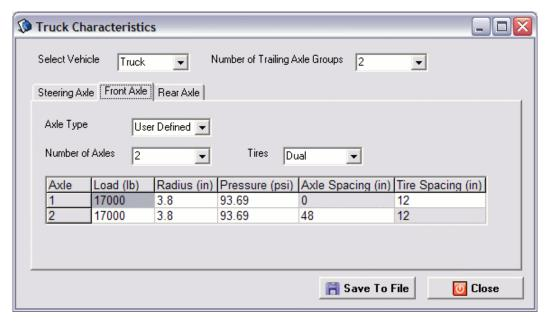
Figure 19 – Truck characteristics.
