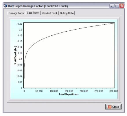
Figure 24 – Rutting vs. load repetitions for each truck.
