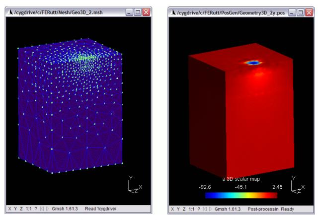
Figure 17 -View mesh (a) and stress contours (b).
