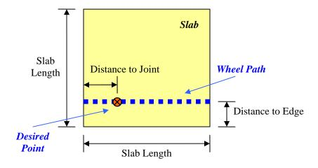
Figure 30 – Wheel path and selected point location within slab.
