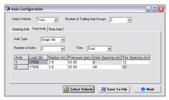
Figure 9 – Axle loading and properties
