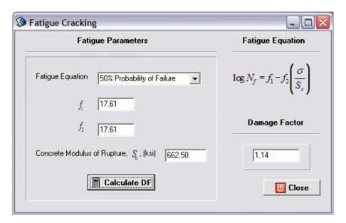
Figure 37 – Available fatigue equations.
