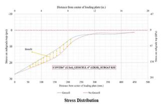
subgrade are reduced at these locations significantly by placing a geocell reinforced layer.
