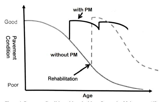
Figure 1. Pavement Condition with and without Preventive Maintenance (68).
