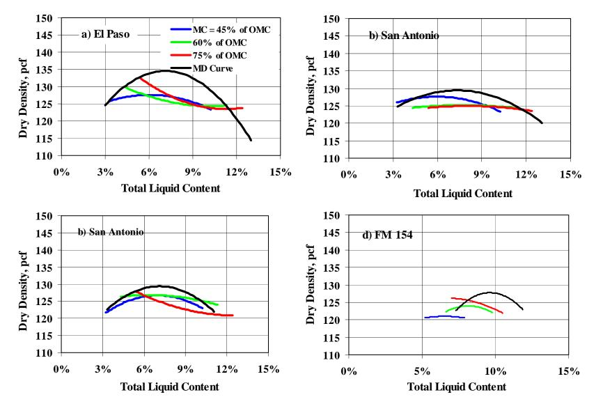
Figure 4.3 – Variations in Density with Total Liquid Content at Different Initial Water Content
