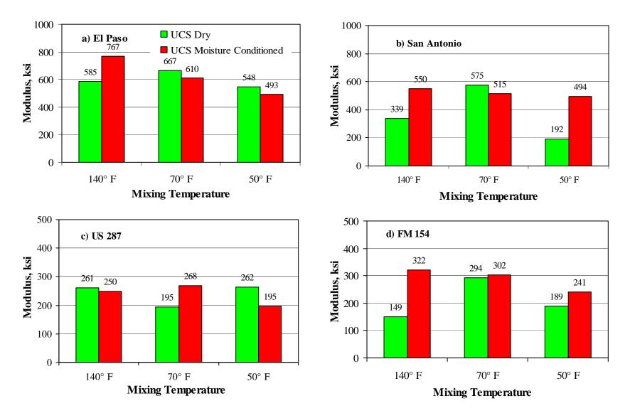
Figure 5.15 – Impact of Mixing Temperature on FFRC Modulus
