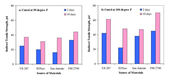
Figure 5.7 – Impact of Curing Time on Indirect Tensile Strength
