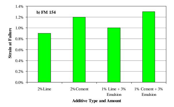
Figure 4.9 – Strains at Failure from Indirect Tensile Strength Tests on El Paso and FM 154 Materials with Different Treatments
