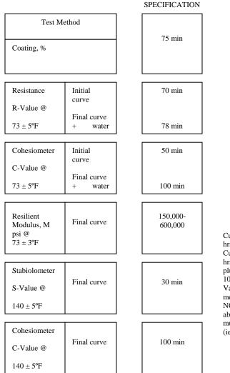
Cured in the mold for a total of 24 hrs. (a) a temperature of  $73 \pm 5^{\circ}$ F. Cured in the mold for a total of 24 hrs. (a) a temperature of  $73 \pm 5^{\circ}$ F, plus 4 days vacuum desiccation at 10-20 mercury.
