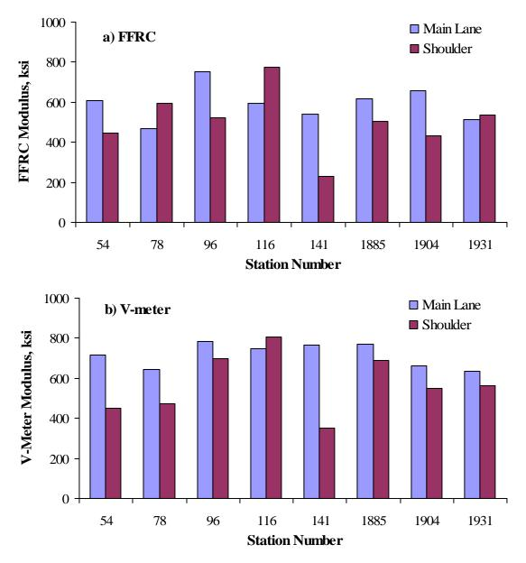
Figure 8.5 – Moduli Measured on UCS Specimens for SH 16 Project
