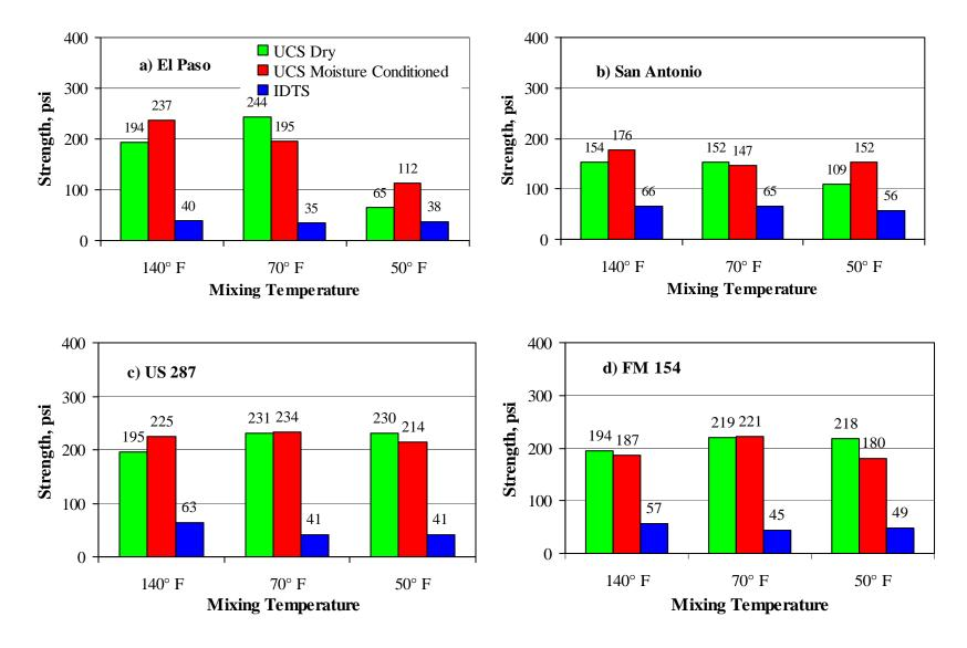
**Figure 5.14 – Impact of Mixing Temperature on Strength Parameters**
