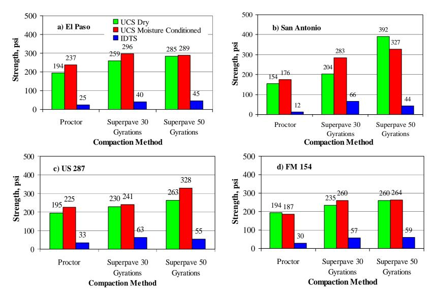
Figure 5.12 – Impact of Compaction Method on Strength Parameters
