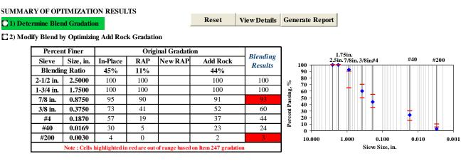
Based on the optimization results, the material required is as follows: - Volume of additional RAP is 0 cubic feet (per linear foot)
