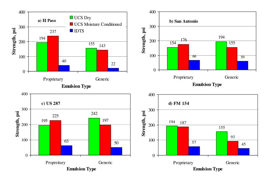
Figure 5.4 - Impact of Emulsion Type on Strength Parameters
