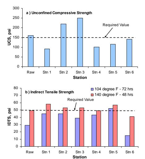
Figure 8.9 – Strengths of Raw and Pulverized Materials from FM 479 Project
