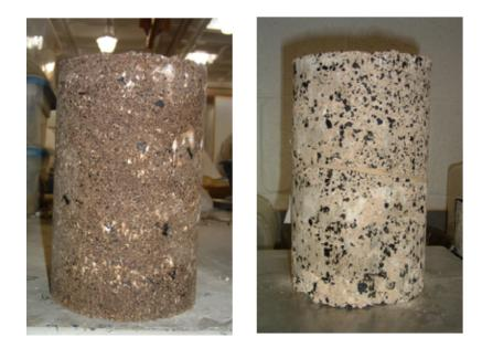
Figure 5.8 – Appearances of Specimens Mixed with High-Shear Mixer (left) and Concrete Mixer (right)
