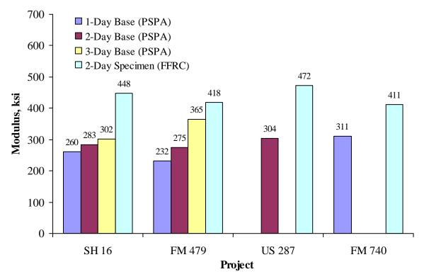
Figure 8.20 – Average Moduli Measured with PSPA and FFRC Device
