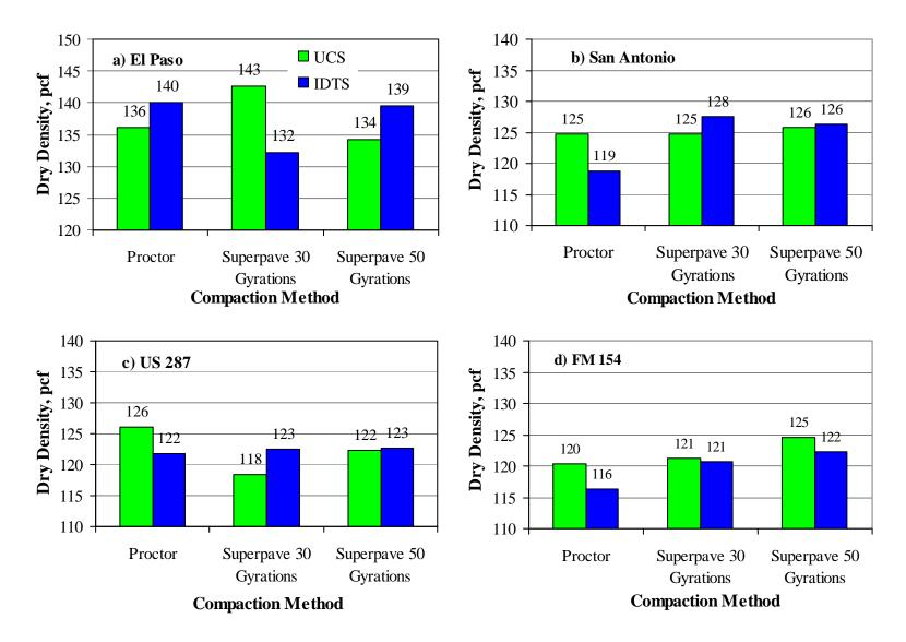
Figure 5.11 – Impact of Compaction Method on Dry Density
