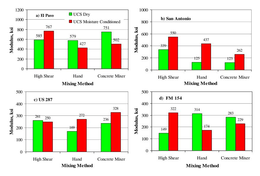
Figure 5.10 – Impact of Mixing Method on FFRC Modulus
