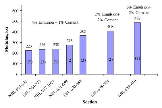
Figure 8.13 – Average Base Moduli from PSPA Measurements for FM 479 Project
