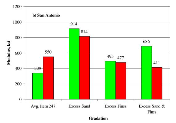
Figure 5.3 – Impact of Gradation on FFRC Modulus
