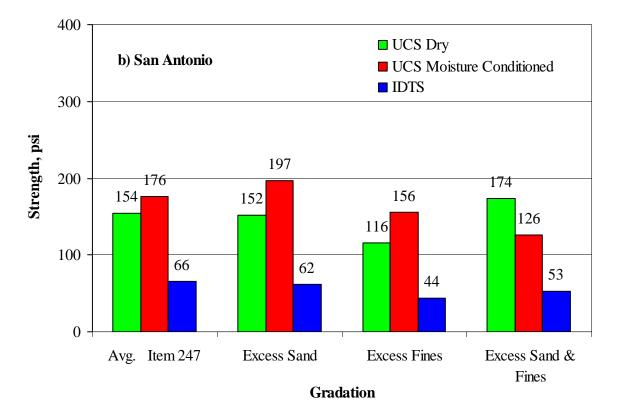
Figure 5.2 – Impact of Gradation on Strength Parameters
