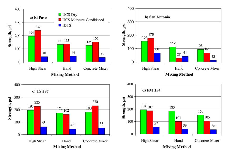
**Figure 5.9 – Impact of Mixing Method on Strength Parameters**
