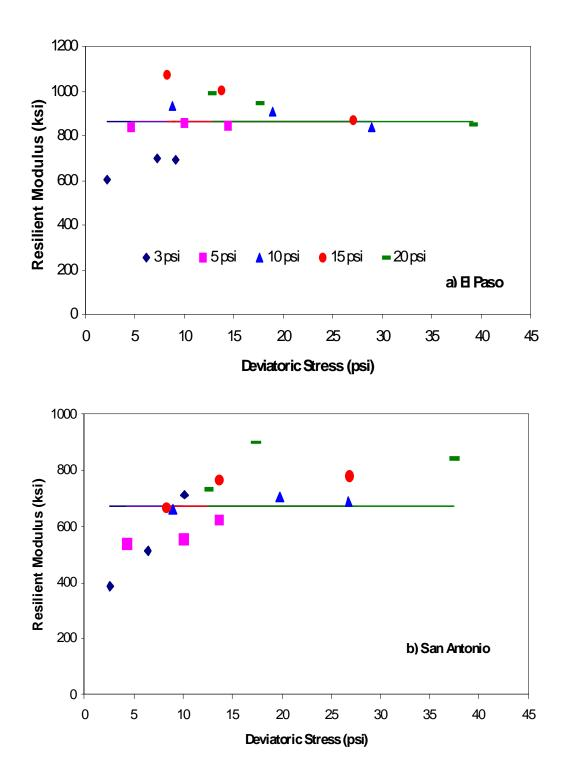
Figure 4.16 – Resilient Moduli of El Paso and San Antonio Materials from Specimens Prepared at Designed Total Liquid Contents
