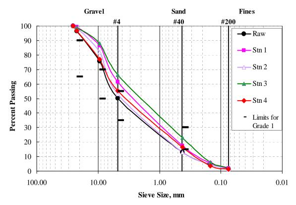
Figure 8.18 – Gradation Curves of Raw and Pulverized Materials from FM 740 Project
