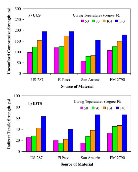
**Figure 5.5 – Impact of Curing Temperature on Strength Parameters**
