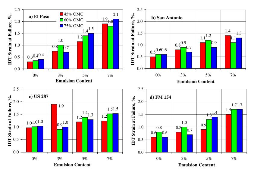
Figure 4.6 - Strains at Failure from IDTS Tests for Materials with Different Moisture and Emulsion Contents
