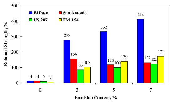
Figure 4.14 – Retained Indirect Tensile Strengths
