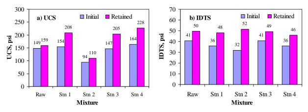
Figure 8.19 – Comparison of Initial and Retained Strengths for FM 740 Project
