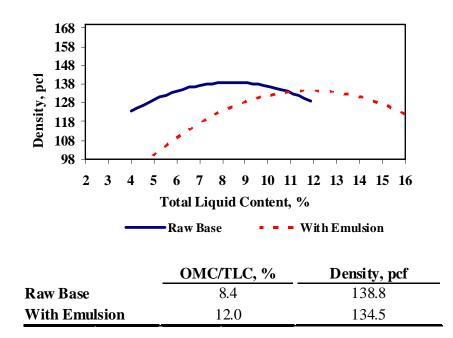
Apparent Moisture Content Vs. Total Liquid Content
