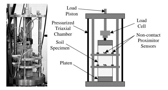
Figure 4.15 – Resilient Modulus Test Device and Setup
