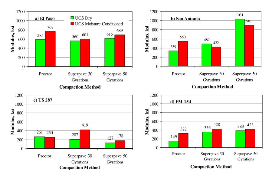
Figure 5.13 – Impact of Compaction Method on FFRC Modulus
