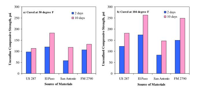
Figure 5.6 – Impact of Curing Time on Unconfined Compressive Strength
