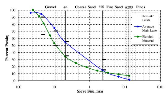
Figure 8.2 – Gradation Curves of Blended Raw Material Used for Mix Design and Material after Pulverization for SH 16 Project
