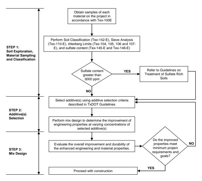
Figure 1 – Flowchart for Subgrade Soil Treatment (from Current TxDOT Guidelines)
