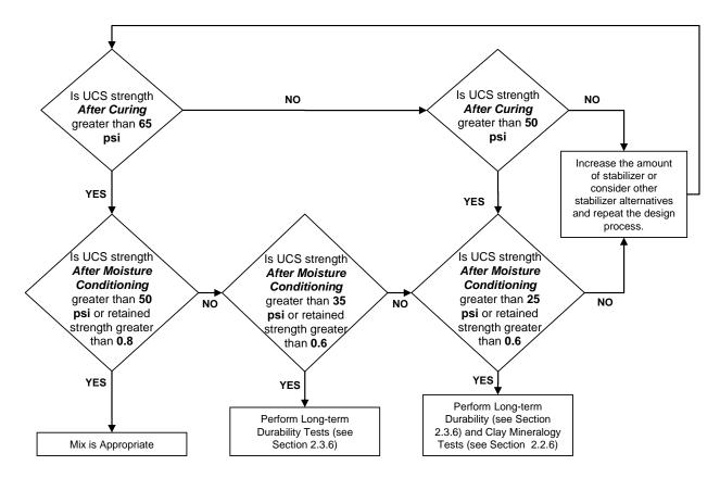
**Figure 4 – Recommended Flowchart to Determine Adequacy of Stabilizer Content**
