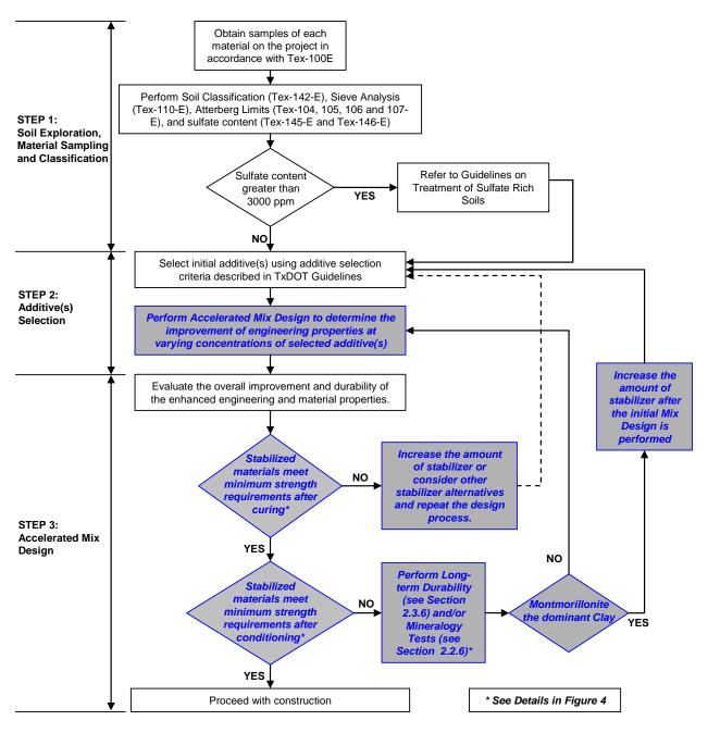
Figure 2 – Proposed Flowchart for Subgrade Soil Treatment
