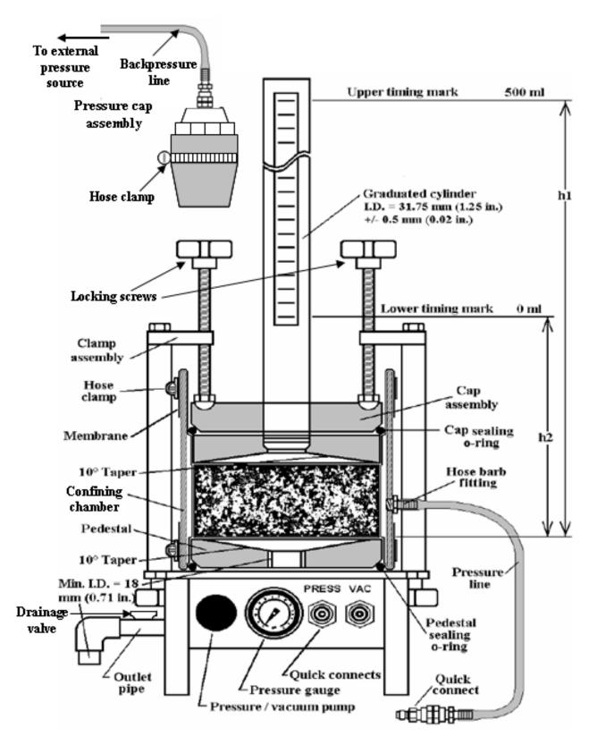
**Figure 1 – Permeability Testing Apparatus**
