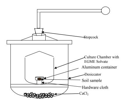
**Figure 1 – Schematic of the Specific Surface Area Apparatus**
