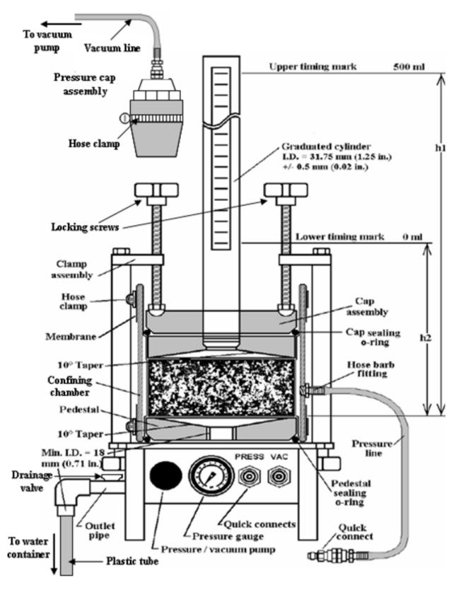
**Figure 2 – Vacuum Testing Apparatus**
