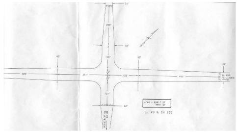
Figure 5.2 - Geometry of SH 155 and SH 49 Intersection.
