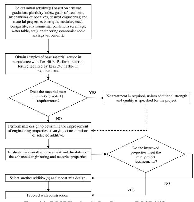
Figure 2.9 - TxDOT Flowchart for Base Treatment (TxDOT, 2005)
