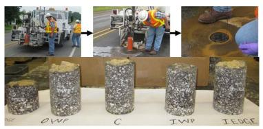
Figure 8.3 - Coring operation for a Core Profile across a Pavement Section.
