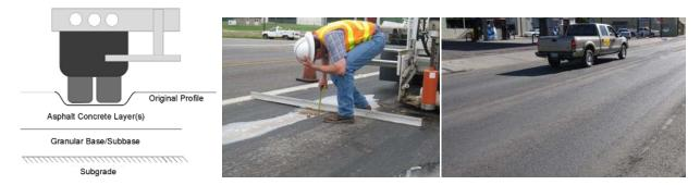
Mechanism: Excessive vertical compressive stresses on the HMA surface causing non-recoverable permanent deformation in the asphalt layer of a pavement structure. Surface rutting will be classified to three levels of severity: a) Low severity is measured less than 0.5 in., b) Medium severity is measured greater than or equal to 0.5 in. and less than 1 in. and c) High severity is measured greater than or equal to 1 in.
