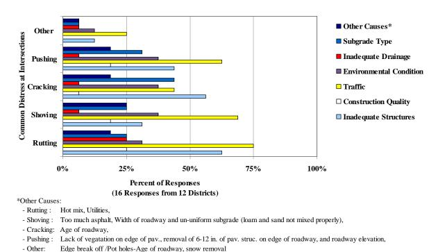
Figure 3.6 – Causes of Distress for Each Type of Distress
