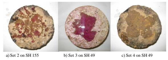
Figure 5.12 - Phenolphthalein Test for Lime on Base Material.
