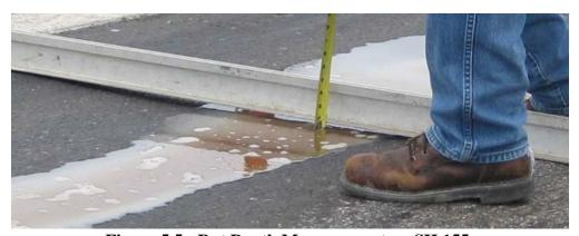
Figure 5.5 - Rut Depth Measurement on SH 155.
