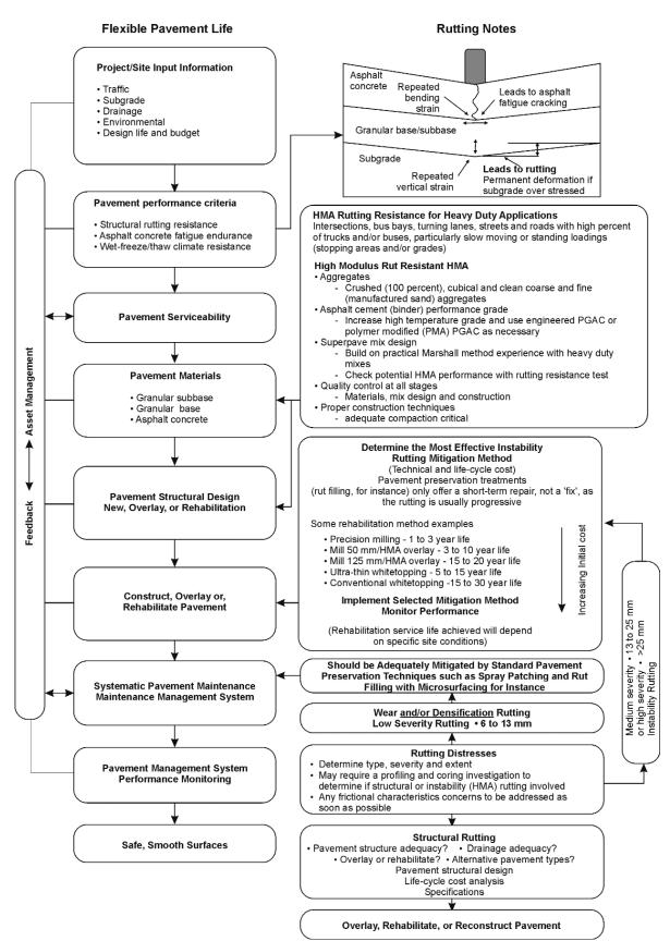
Figure 2.8 - Flowchart of Activities for Mitigating Intersection Rutting.
