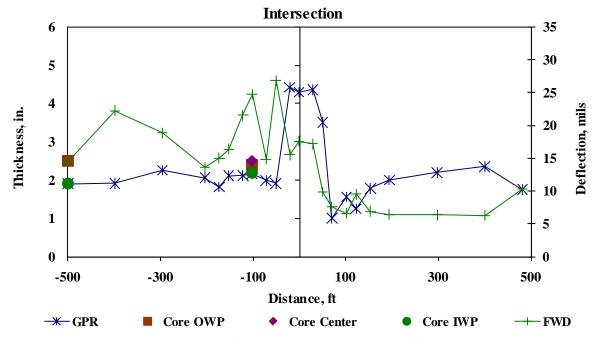
Figure 5.16 - GPR, FWD and Cores on SH 155.
