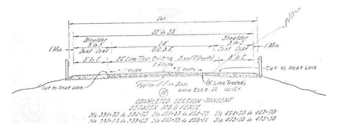
b) SH 49 Pavement Figure 5.3 - Cross-sectional Pavement Design for SH 155 and SH 49
