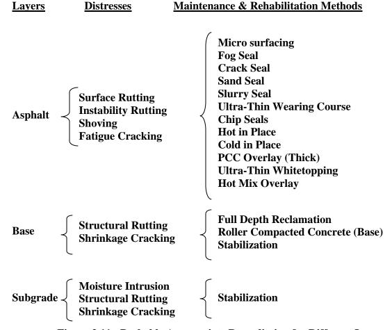
Figure 2.11 - Probable Appropriate Remediation for Different Layers
