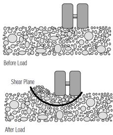
Figure 8.4 - Illustration of Instability Rutting.
