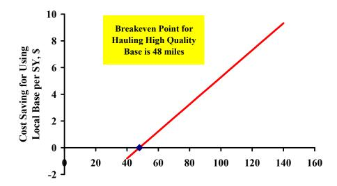
Figure 5.17 – Worksheet of Cost Analysis for Roadway Base Construction with Low and High Quality Materials
