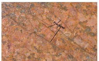
Figure A.12 - Polished Slab of Granite
