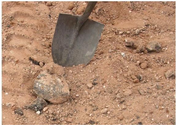
Figure 5.7 - Large-size HMA after pulverization
