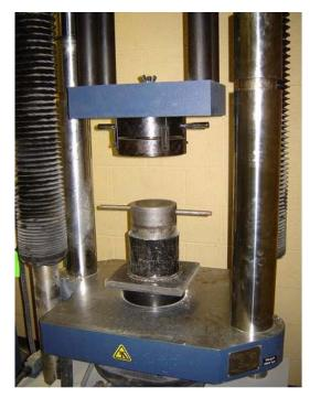
Figure 5.3 – ACV and AIV Testing Apparatus
