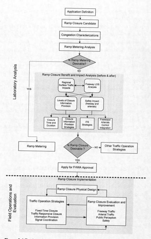
Figure 2-1 Engineering Analysis Procedure for Peak-Period Ramp Closure
