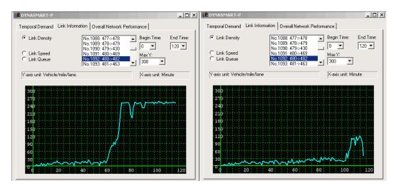
Figure 2-5 DYNASMART-P Link Statistics Comparison between Scenarios
