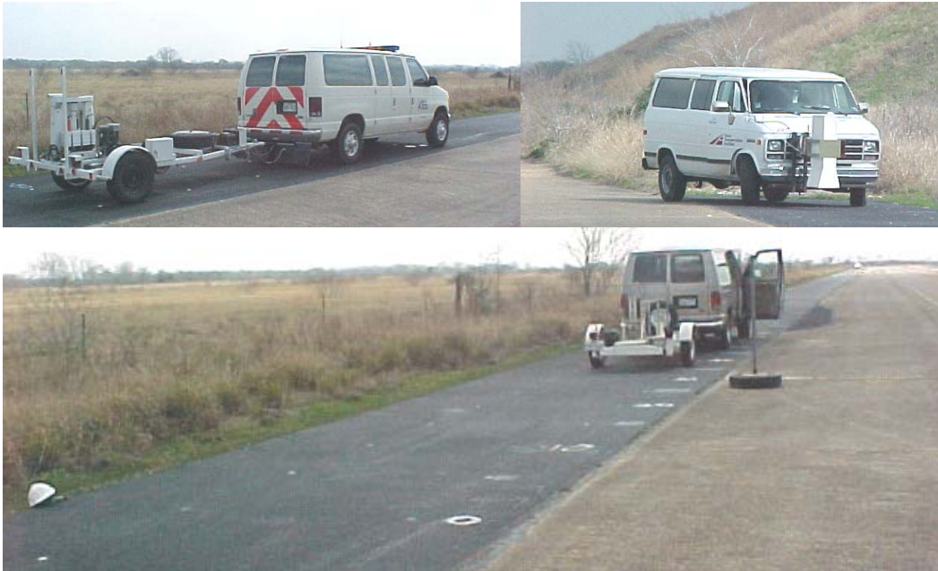
Figure 4.4 - FWD, SPA, and GPR Data at the TTI Test Site
