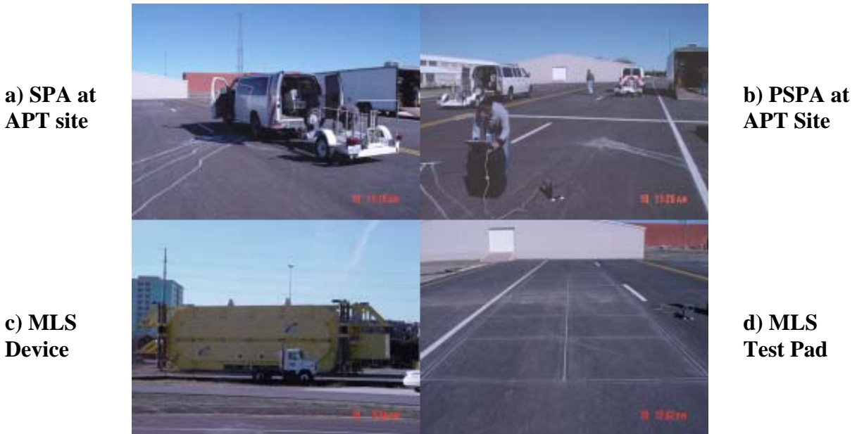
Figure 4.7 - Pictures of the NDT Devices and MLS Pad at APT Site
