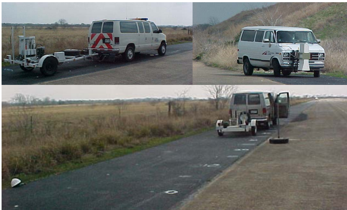
Figure 5.9 - FWD and SPA at the Ride Rut facility
