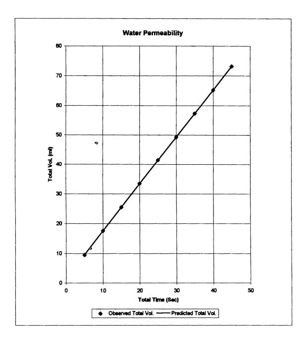
Figure 2. Permeability of Specimen Consisting of 3% Cement, 75/25 Flyash-Sand Ratio With Water-Cement Ratio of 3.00
