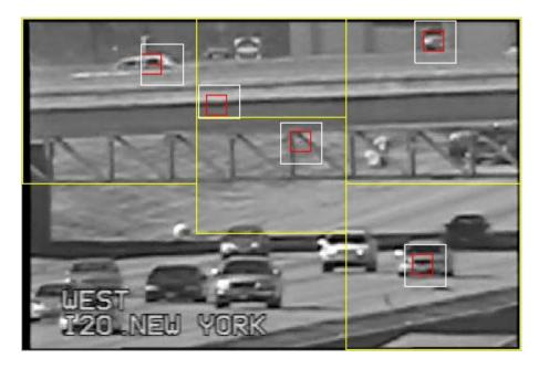
Figure 5.6 Selected targets with maximum standard deviation in each block.
