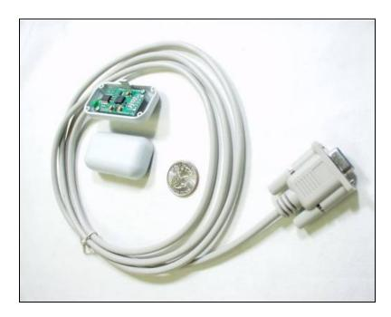
Figure 4.15 Tri-Axis serial accelerometer.
