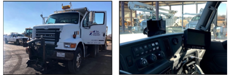
Figure 1. A TxDOT snowplow with a mounted tablet on the front windshield
