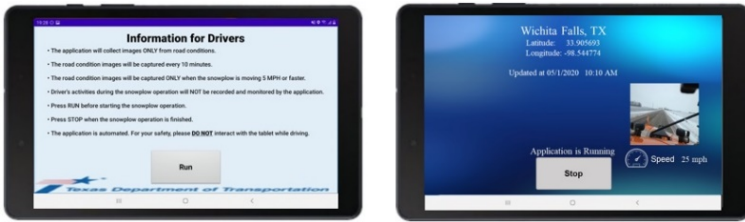
Figure 2. Custom application running on a tablet to collect road condition images
