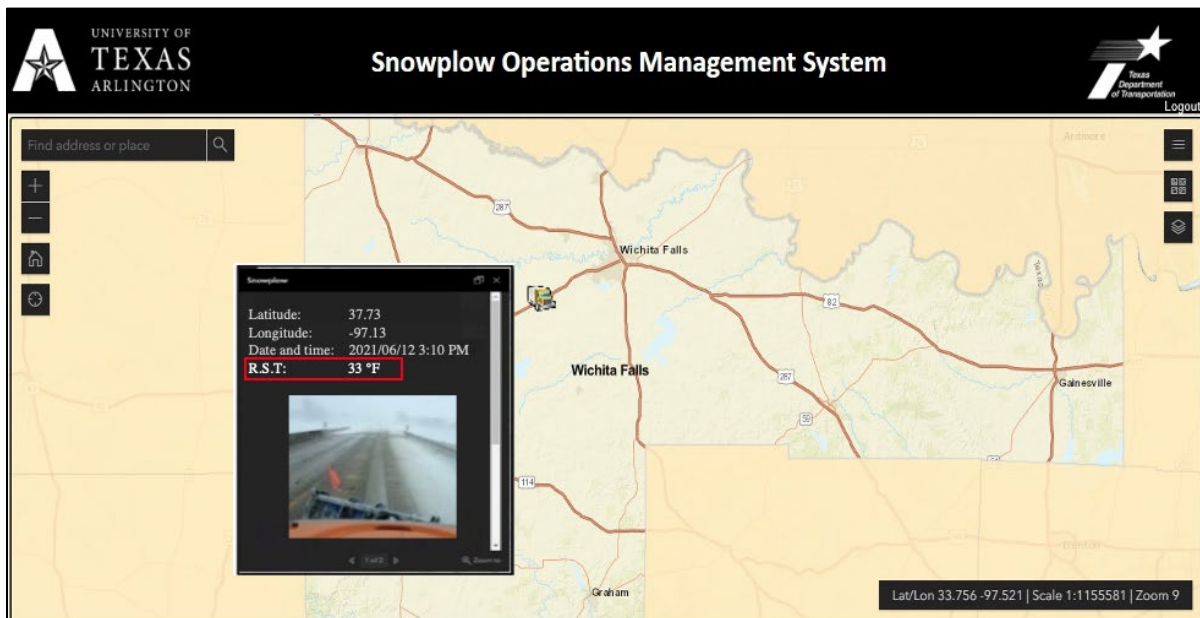
Figure 4.6 Schematic view of the map-based interface displaying the actual road surface temperature, collected by the temperature sensor, along with snowplow location
