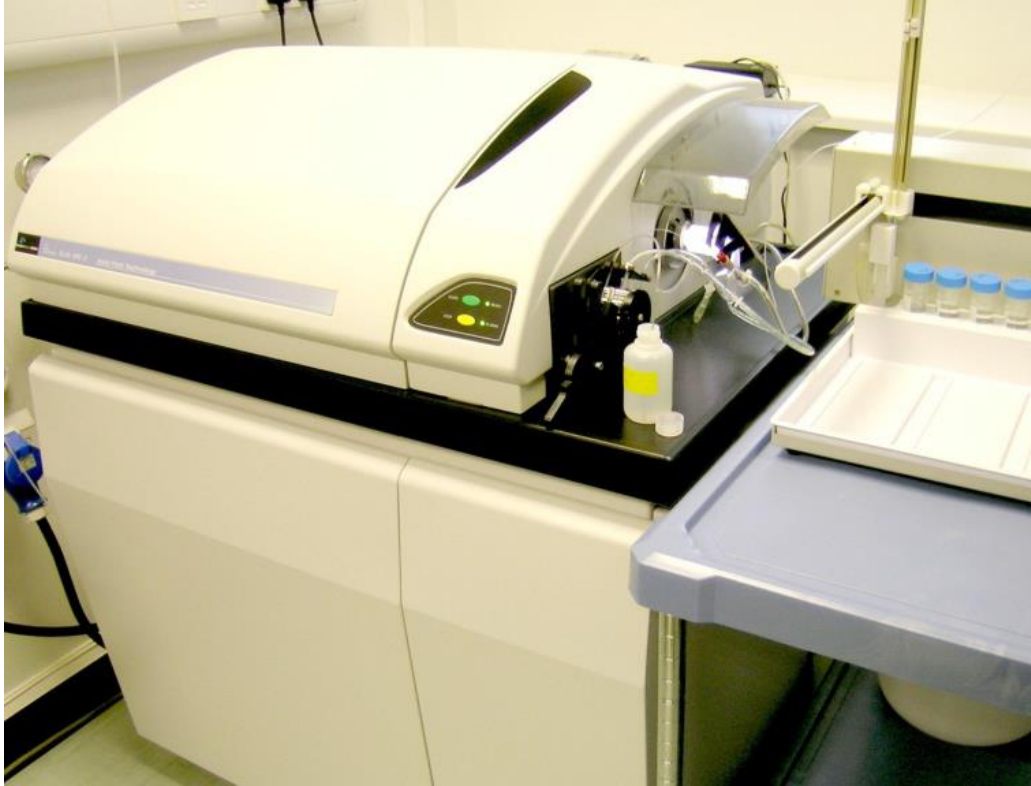
Figure 34: ICP-MS instrument for determination of Silica and Alumina levels
