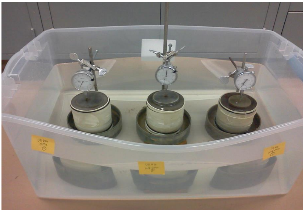
Figure 32: Three Dimensional Swell test
