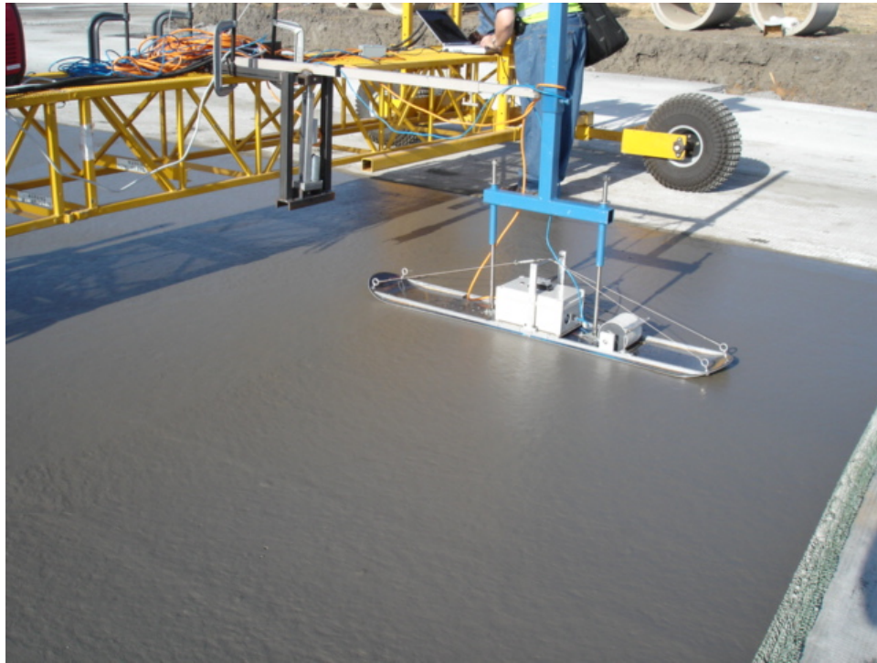
Figure 6 Sliding Profiler Attached to a Motorized Work Bridge
