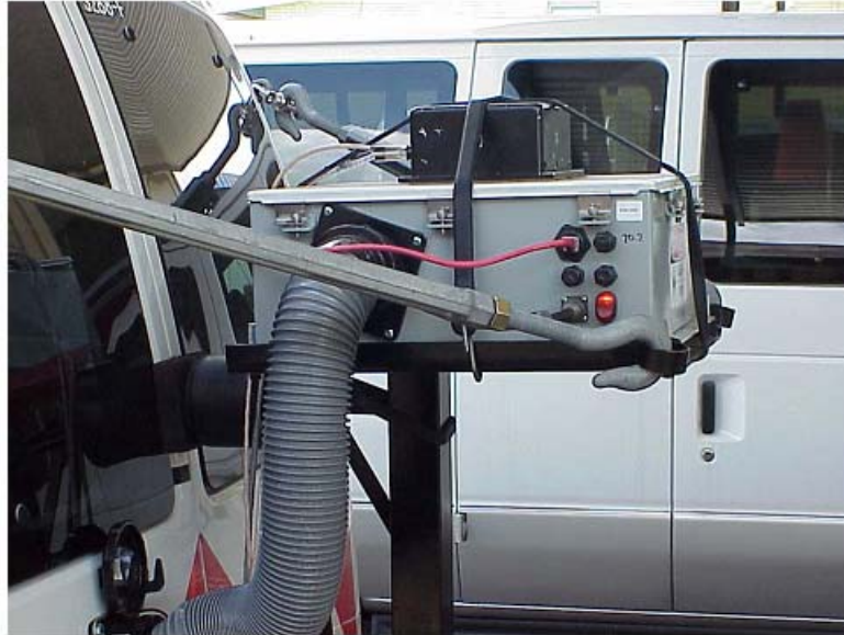
Figure 6 Scanning Laser System Shown with External Cooling on TxDOT TMV
