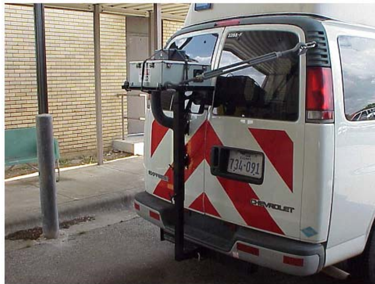
Figure 5 Scanning Laser System Mounted on TxDOT TMV
