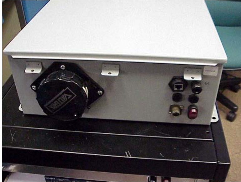
Figure 4 TxDOT Scanning Laser System Ready To Install on Vehicle
