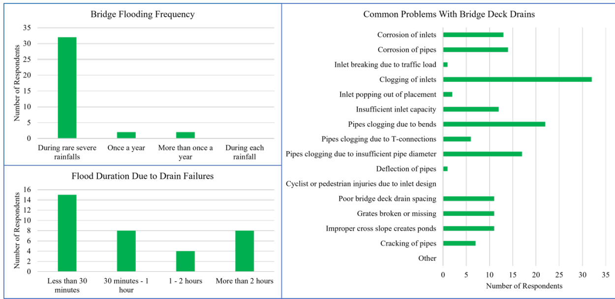
Figure 3.4 Summary of survey responses on bridge deck drain failure (outside Texas)
