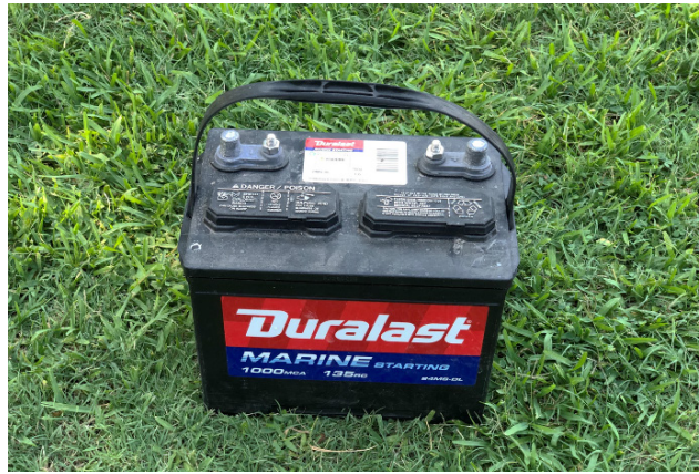
Figure 3.11 External marine 12 V battery
