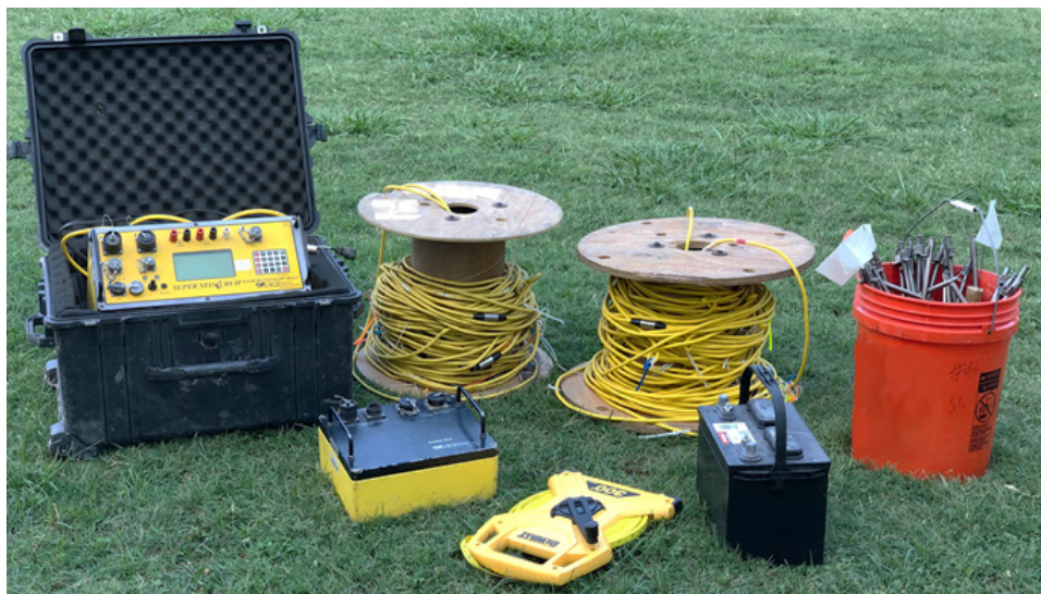
Figure 3.6 Required equipment for the implementation of an electrical resistivity survey in the field
