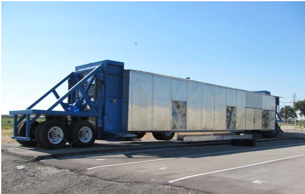
Figure 3.6. PTM Placed on Top of Rutting Sections J and K.
