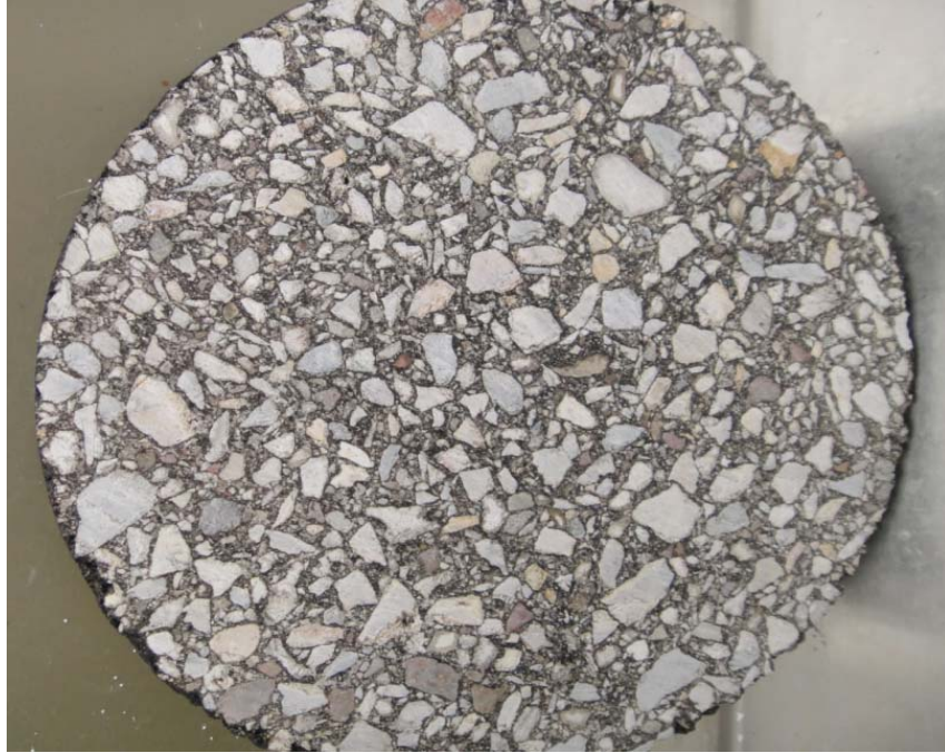
Figure 4.1. Cut Face of the 20 Percent RAP Mix.
