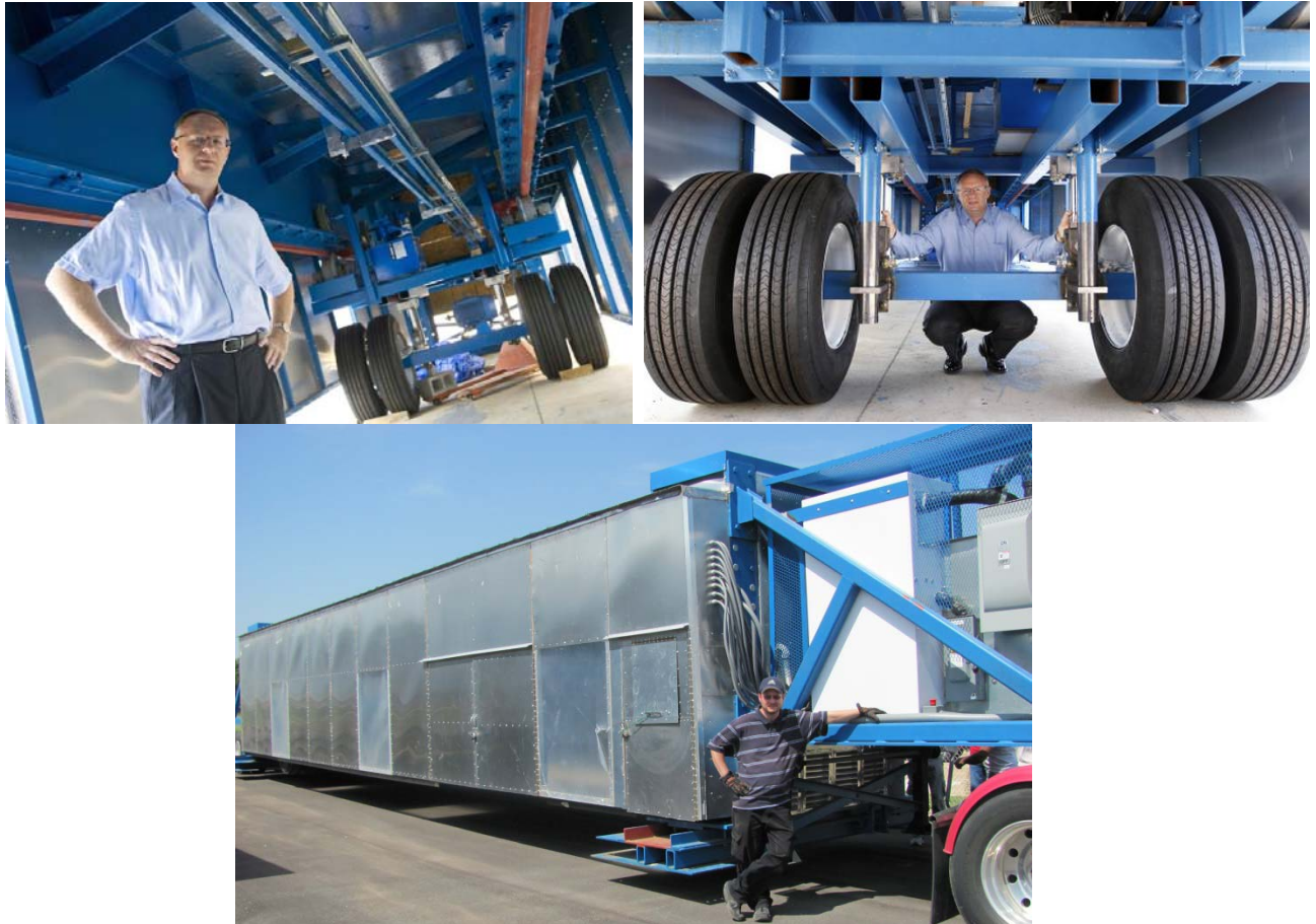
Figure 3.5. Photos of the Pavement Testing Machine.
