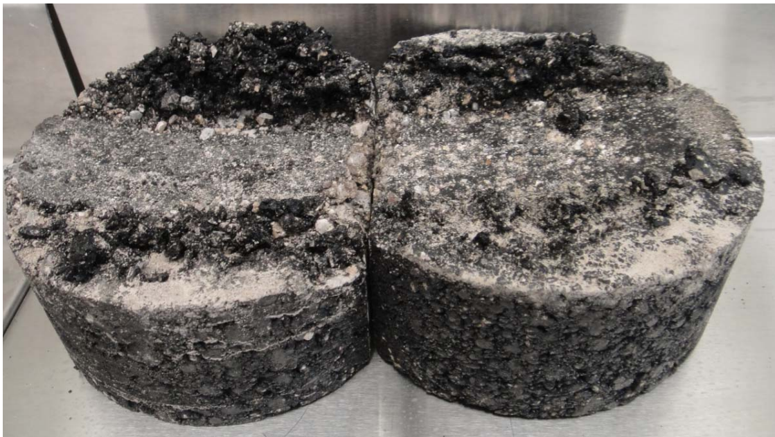
Figure 4.2. Control Mix after Testing—Many Fines Stripped Out.
