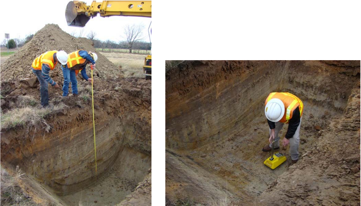
Figure 3.2. Soil Sampling and Density Measurement by Using Nuclear Gauge.
