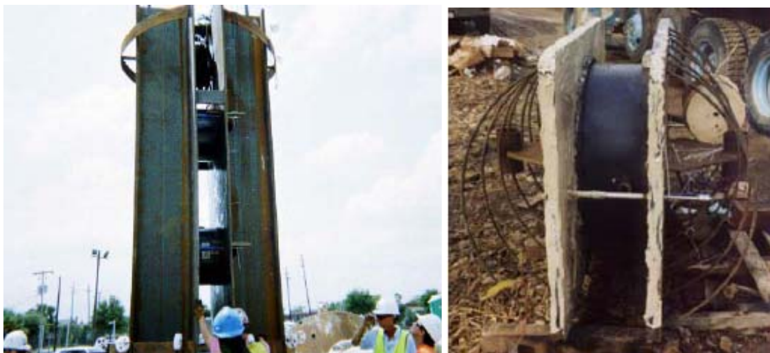
Figure 2.23. Osterberg Load Cell for the Lateral Load Test. (Source: http://www.loadtest.co.uk/Loadtest%20Ltd/downloads.htm )
