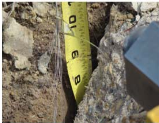
(c) Soil-Test Shaft Separation (Depth)
