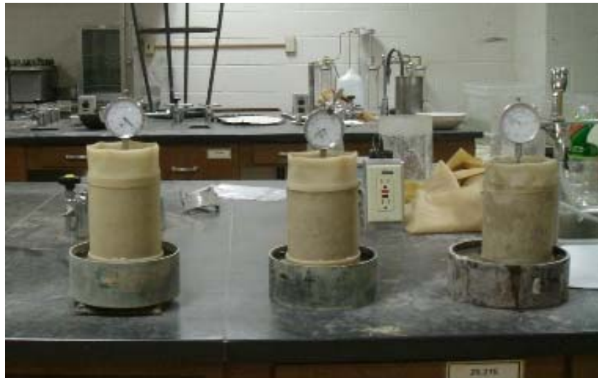
Test Setup of 3D Swell Test (Dry OMC, OMC, and Wet OMC [left to right])
