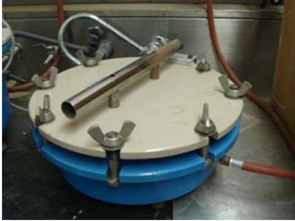
Figure 3.17. Pressure Plate Testing.
