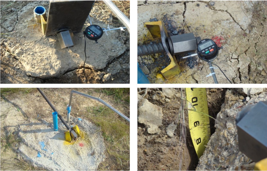
Figure 5.8. Test Shaft Displacements in Summer Condition.
