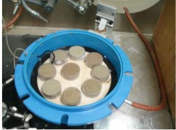
Figure 3.17. Pressure Plate Testing.
