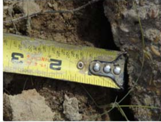
(b) Soil-Test Shaft Separation (Distance)
