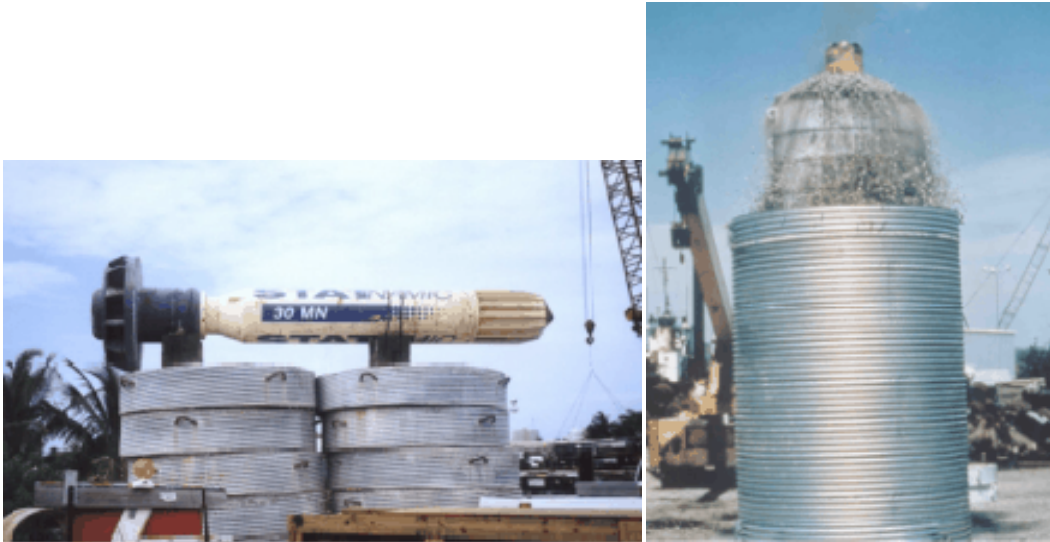
Figure 2.24. Test Setup for a Statnamic Test.
