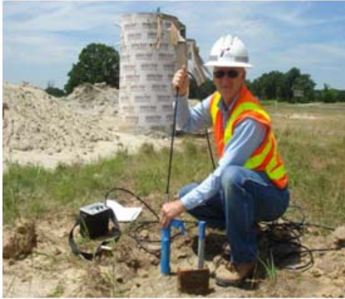
Figure 4.15. Taking Initial Inclinometer Readings.
