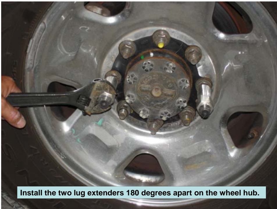
Figure 33 Mounting Lug Extenders
