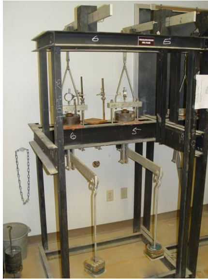
Figure 3.5 Constant volume swell pressure test setup
