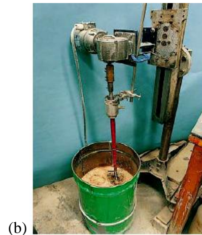
Figure 2.11 Domestic dough mixer and mixing blades (JGS 0821-2000)
