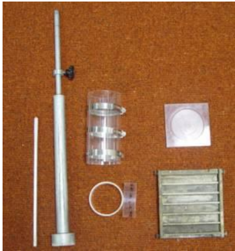
Figure 3.9 Details of compaction rammer, poking rod, free swell mold, UCS mold, base plate and linear shrinkage mold
