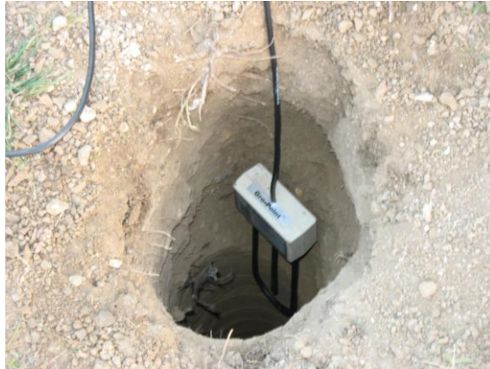
Figure 5.33 Field schematic of Gro-Point moisture probe installation
