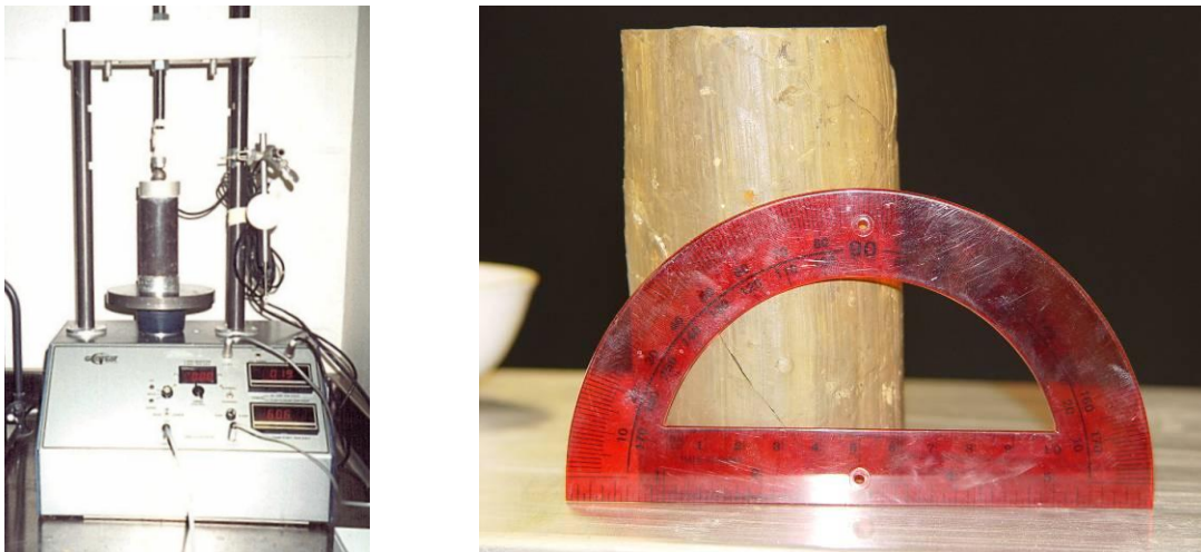
Figure 3.7 (a) UCS test set-up (b) Shear failure of specimen
