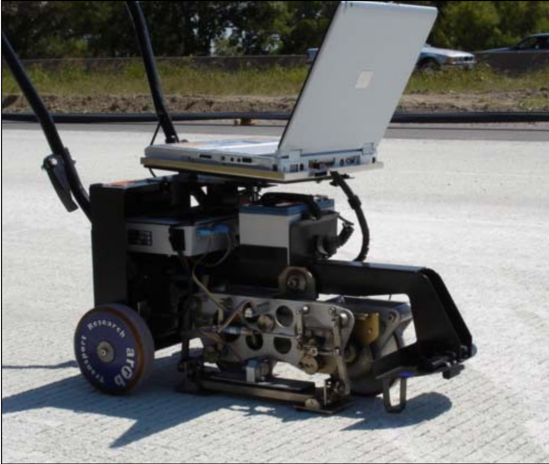
Figure 3.13. Walking Profiler Used to Collect Reference Elevation Measurements.
