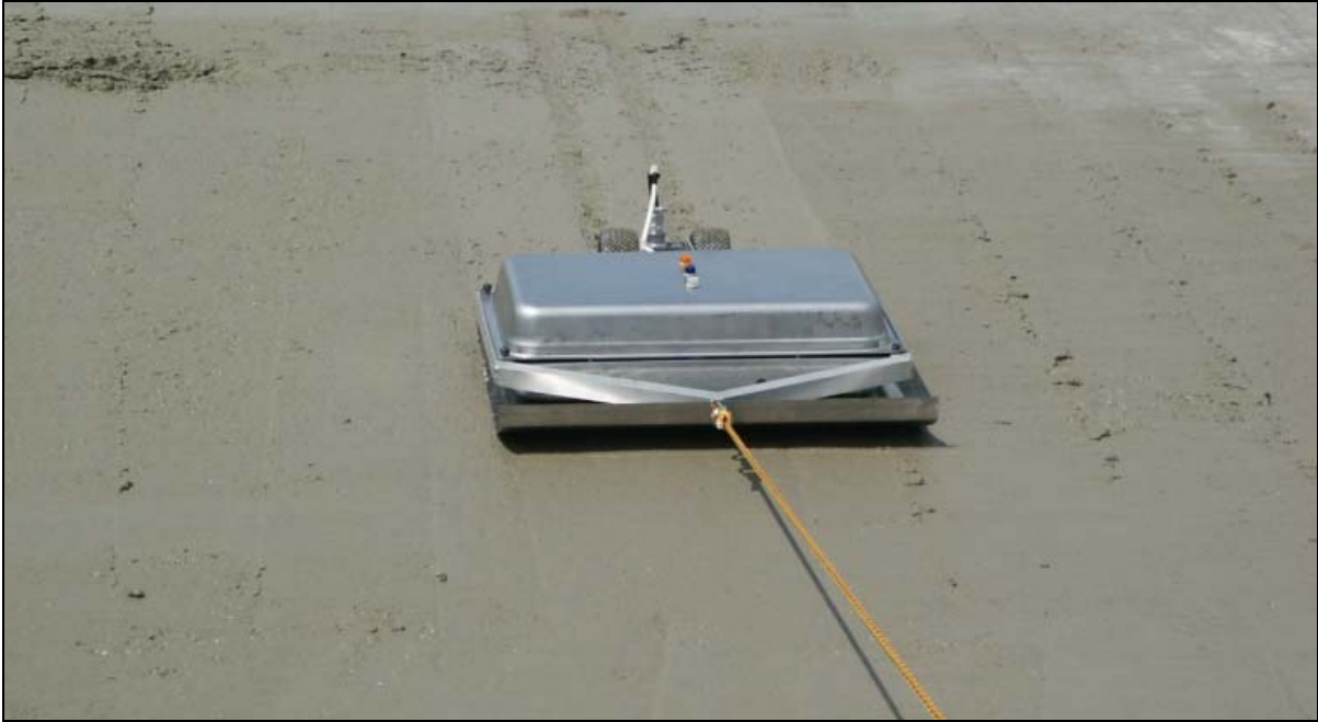
Figure 3.6. Test on Fresh Concrete with Sliding Profiler on Sled.
