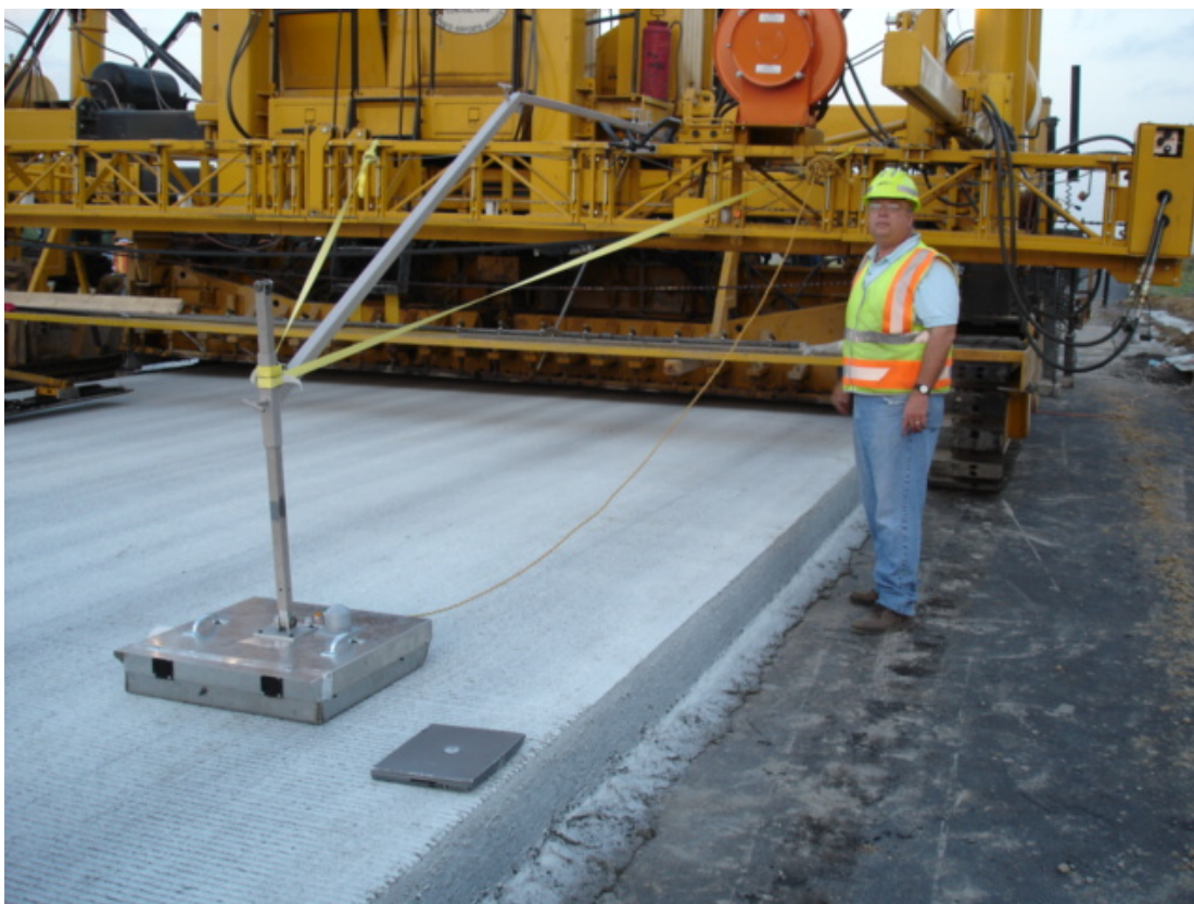
Figure 3.9. Prototype Sliding Profiler Tested on I-20 Project.
