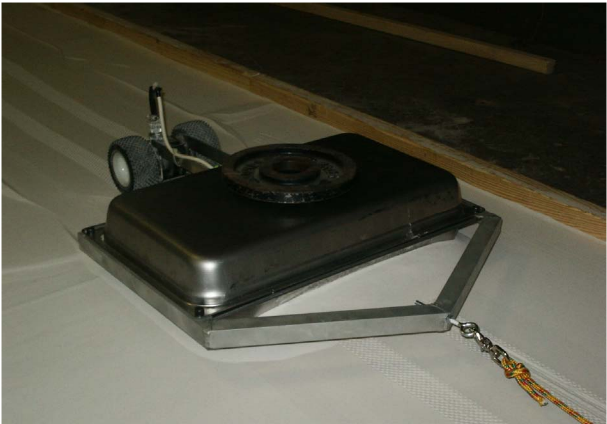
Figure 3.5. Sand Box Testing of Initial Sliding Profiler.
