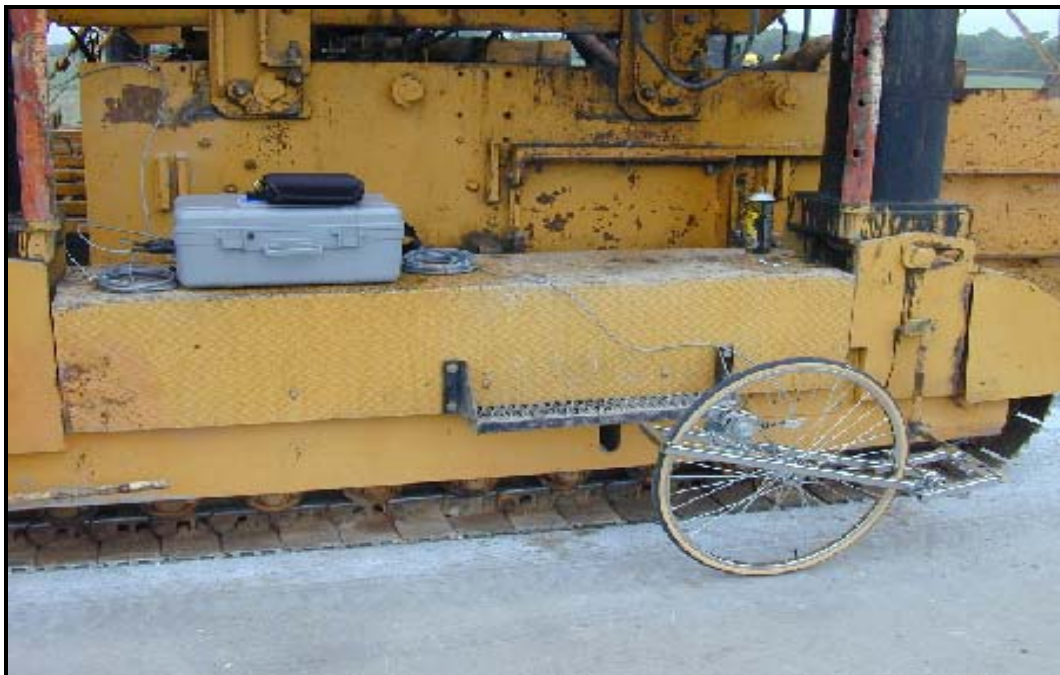
Figure 13. Fifth Wheel Used to Measure Distance in Real Time Profiler.
