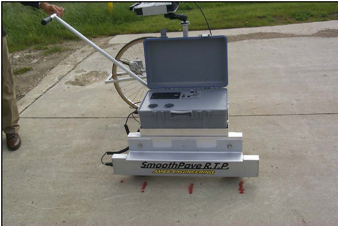
Figure 1. Picture of Ames Real Time Profiler (red painted lines on pavement indicate locations of three lasers).
