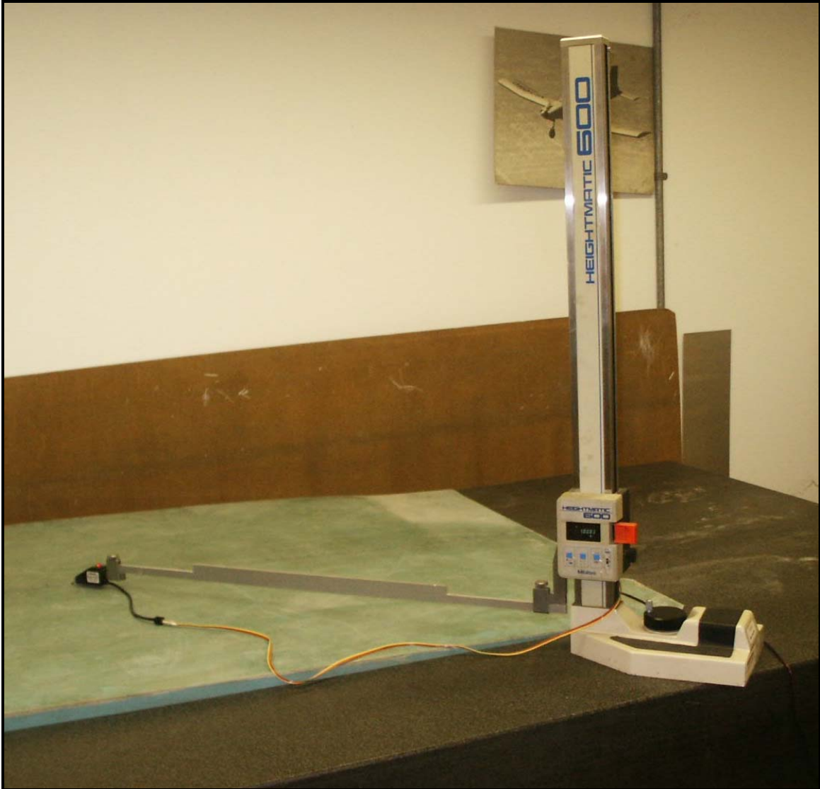
Figure 4. Measuring the Bump Profile in the Laboratory.
