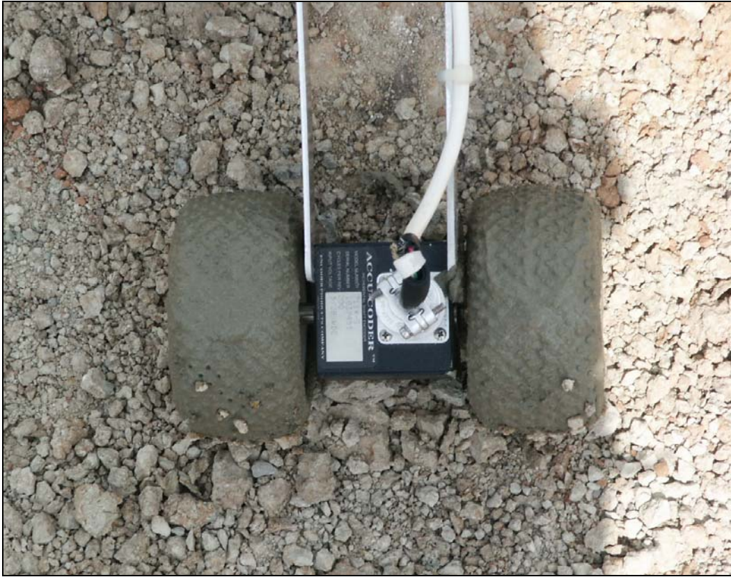
Figure 3.7. Concrete on Measuring Wheels.
