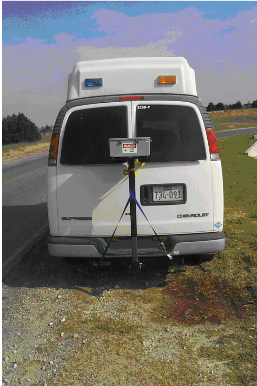
Figure 3.8 Scanning Laser Mounted on TxDOT Test Vehicle
