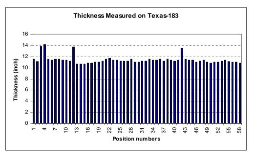
Figure 4.3 Measured thickness on Texas 183 southbound.
