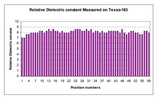
Figure 4.4 Measured dielectric constants on Texas 183 southbound.
