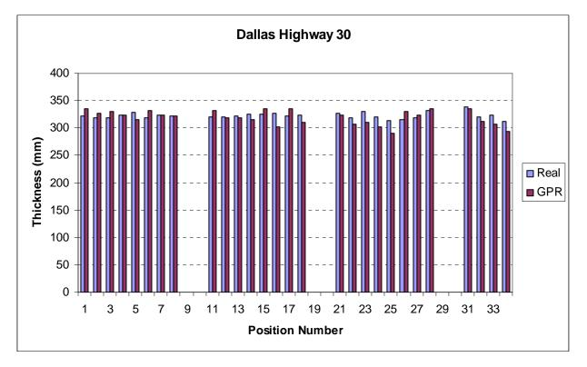
Figure 4.2 Comparison of the GPR measured thickness with real thickness on Highway 30, Dallas.
