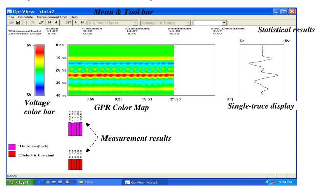
Figure 2.3 GPR software interface.
