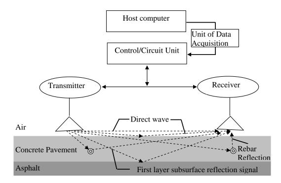
Figure 2.1 Block diagram of the CPT-GPR system.
