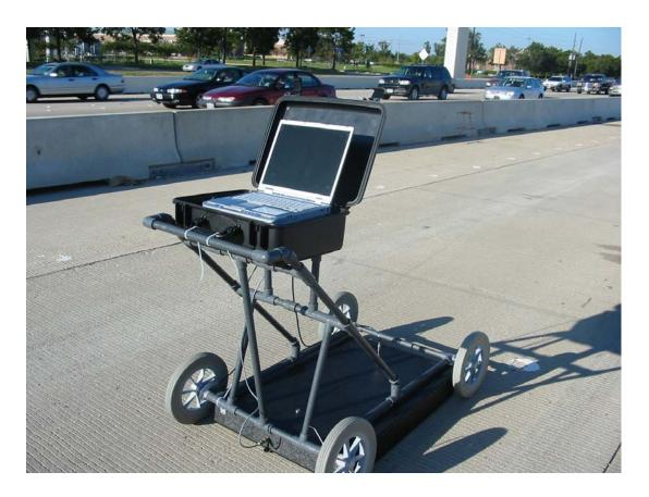
Figure 2.2 GPR system in measurement configuration.
