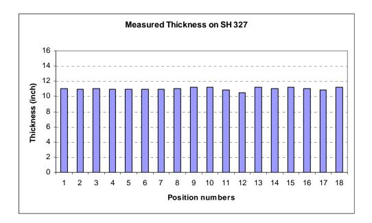
Figure 4.5 Measured thickness on SH 327.
