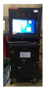
Fig. 3-6: HBM Spider 8 data acquisition system.
