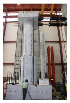
Fig. 2-10: Tests on column-oversized drilled shaft assemblies.
