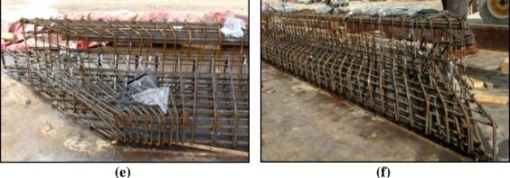
Figure 3.5. Partial Reinforcing Details of Phase 2 Specimens: (a) Specimen ITBC-30-T-M, (b) Specimen ITBC-30-S-M, (c) Specimen ITBC-45-T-M, (d) Specimen ITBC-45-S-M, (e) Specimen ITBC-60-T-M and (f) Specimen ITBC-60-S-M
