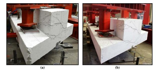
Figure 4.53. Torsional cracking profile at peak load : (a) ITBC-45-T-2M and (b) ITBC-45-S-2M
