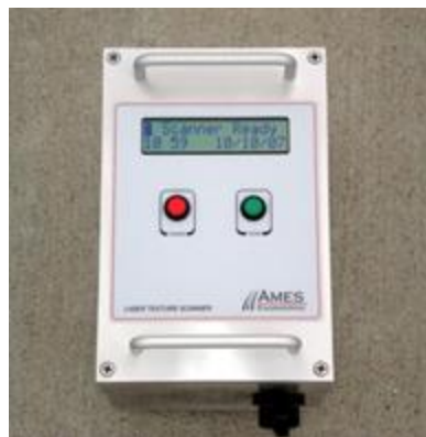
Figure 13. Laser Texture Scanner
