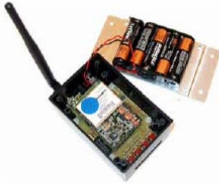
Figure 34 Wireless MEMS sensor in the Geumdang Bridge (after J. P. Lynch et al. [58])
