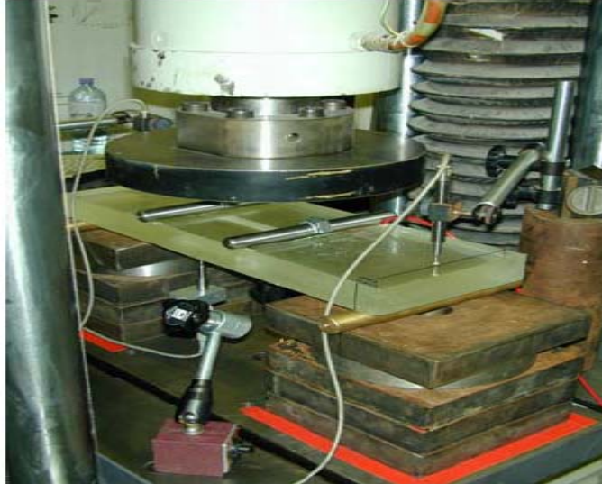
Figure 9 Test zone of the four-point-bending setup (after M. Heinrich and M. Janaushek [35])
