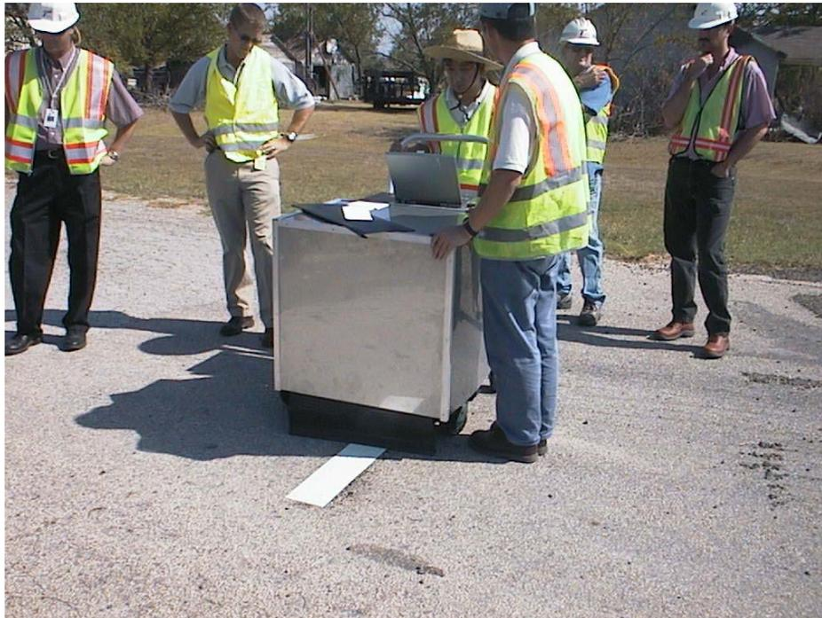
Figure 5.7. (a) Field-test in Waco District – TPMM over old asphalt pavement
