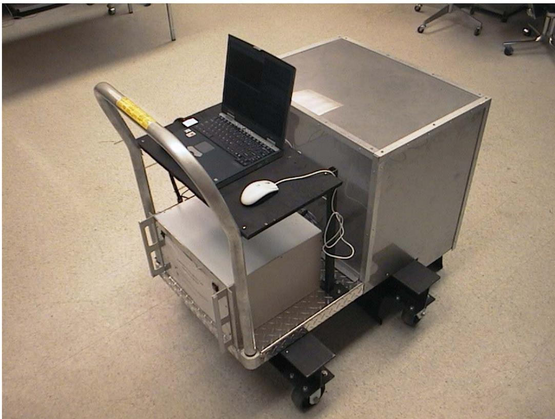
Figure 2.3 Prototype device for thermoplastic thickness measurement
