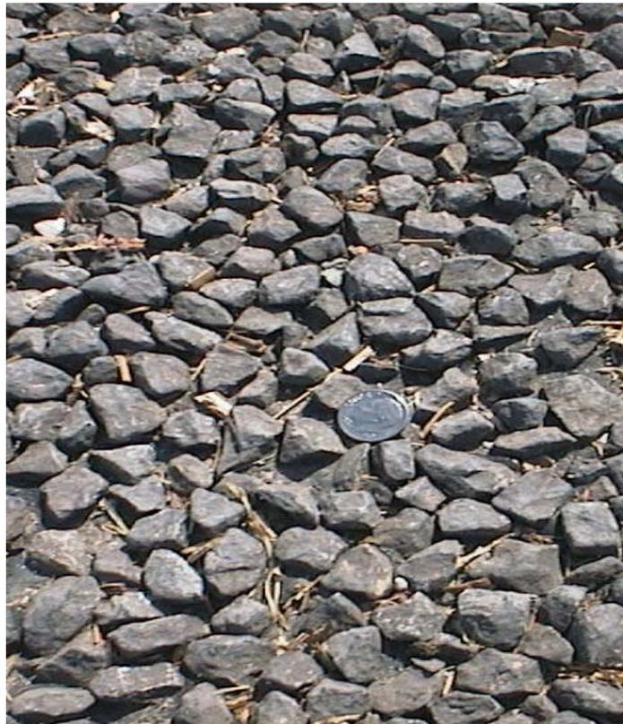
Figure 5.8 (c) Relative gravel size used in Waco new pavement
