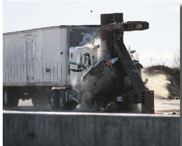
80,000-lb Tractor-Trailer Impacting Simulated Bridge Pier
