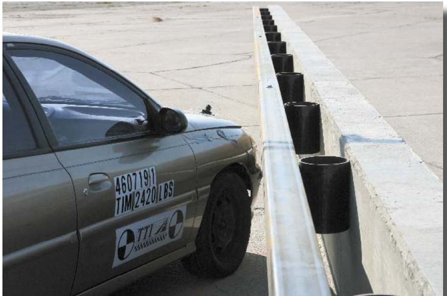
Figure 1. Photograph of High-Speed Energy-Absorbing Bridge Rail with passenger Vehicle.
