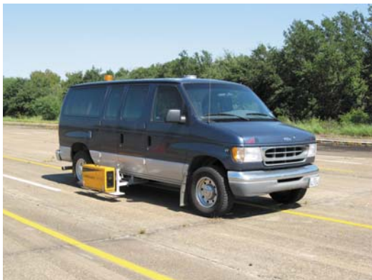
Figure 1. Mobile retroreflectivity unit mounted to vehicle.
