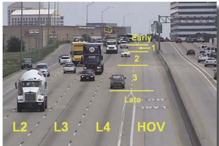
Division of Access Opening and Lane Assignments at Example Site
