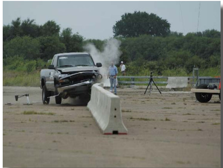
Crash Test of Texas Precast Concrete F-Shape Barrier with Type X Connection Using a 5000-lb, ¾-ton Pickup.
