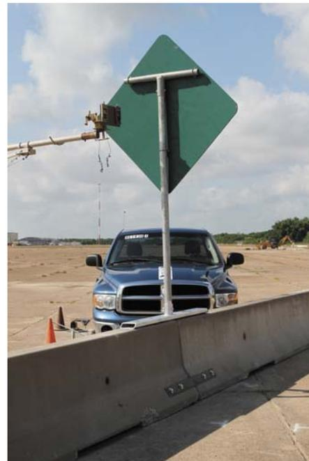
**Figure 2: Impact Angle of Test Vehicle with the Sign Support Assembly.**
