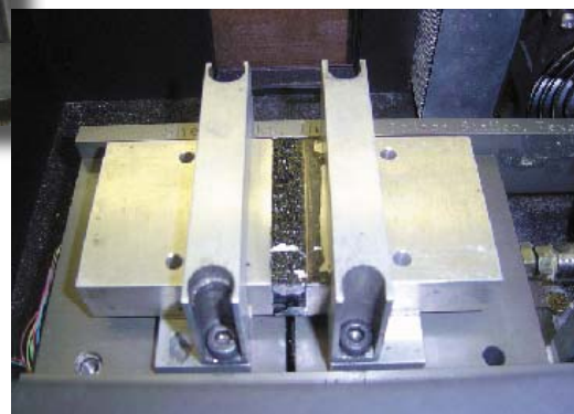
Overlay Tester-based Crack Sealant Adhesion Tester.
