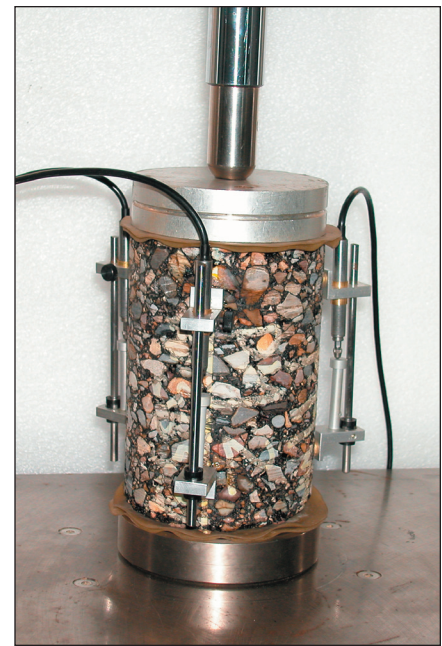
Figure 1. Setup for Simple Performance Tests (Dynamic Modulus, Flow Time, and Flow Number).
