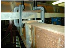
Figure 4 Connection between braces and girder top flange
