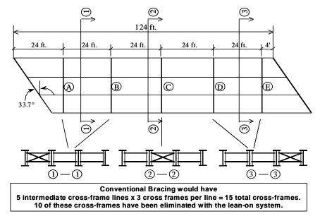
Figure 5 Proposed layout of cross-frames with lean-on bracing
