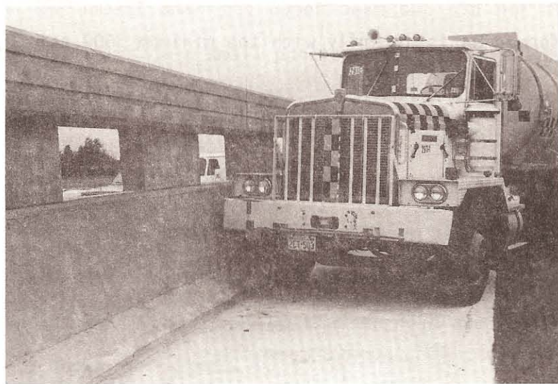
Figure 4. Comparison of Thunderbird and 80,000 lb Tank Truck with Modified Rail
