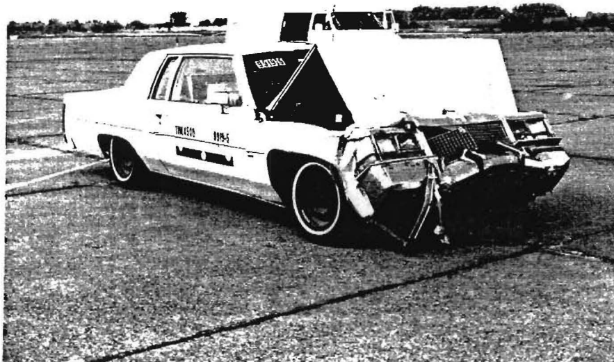
Figure 14. Vehicle after impact with Energy Absorption TMA.
