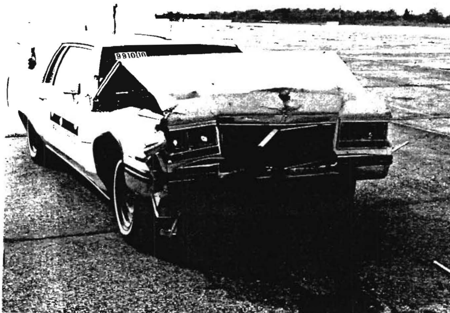
Figure 99 Vehicle after impact with Connecticut TMA (9910-10).
