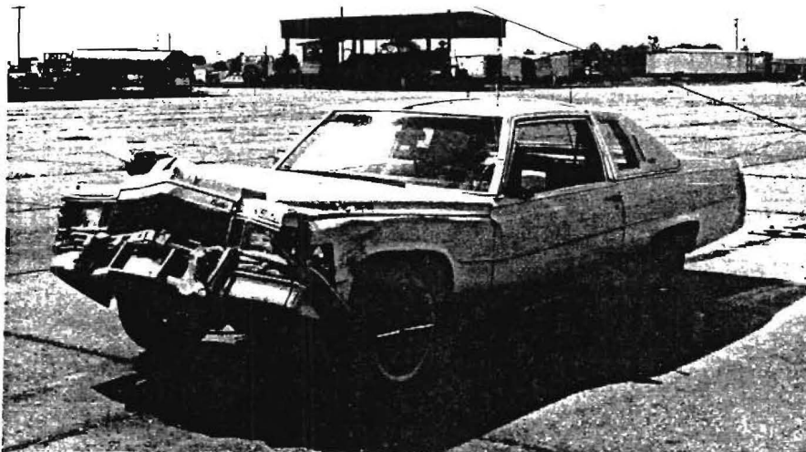
Figure 51. Test vehicle after impact with Hexcel Tx-4000 TMA.
