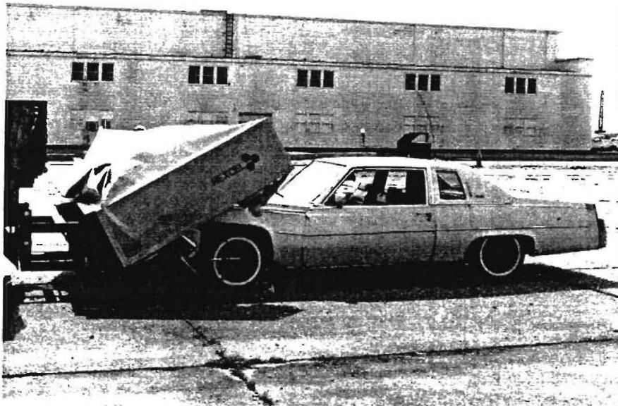
Figure 50. Damage to Hexcel Tx-4000 TMA (left side).
