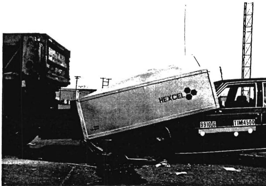
Figure 61. Hexcel Model 4000 TMA after test 9910-6.
