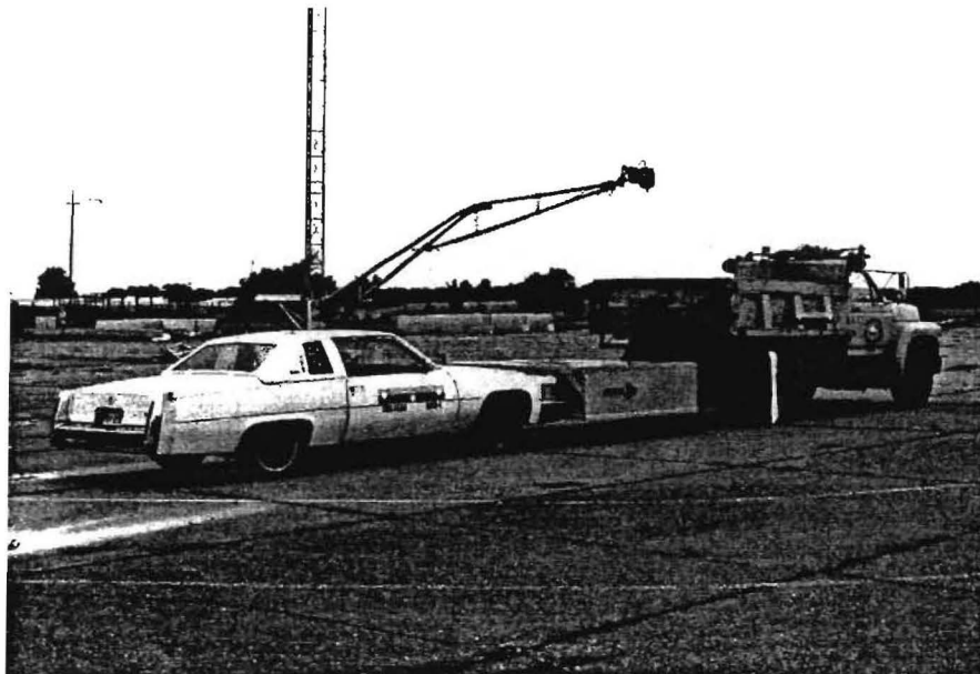
Figure 45. Configuration for test with Hexcel Tx-4000 TMA.
