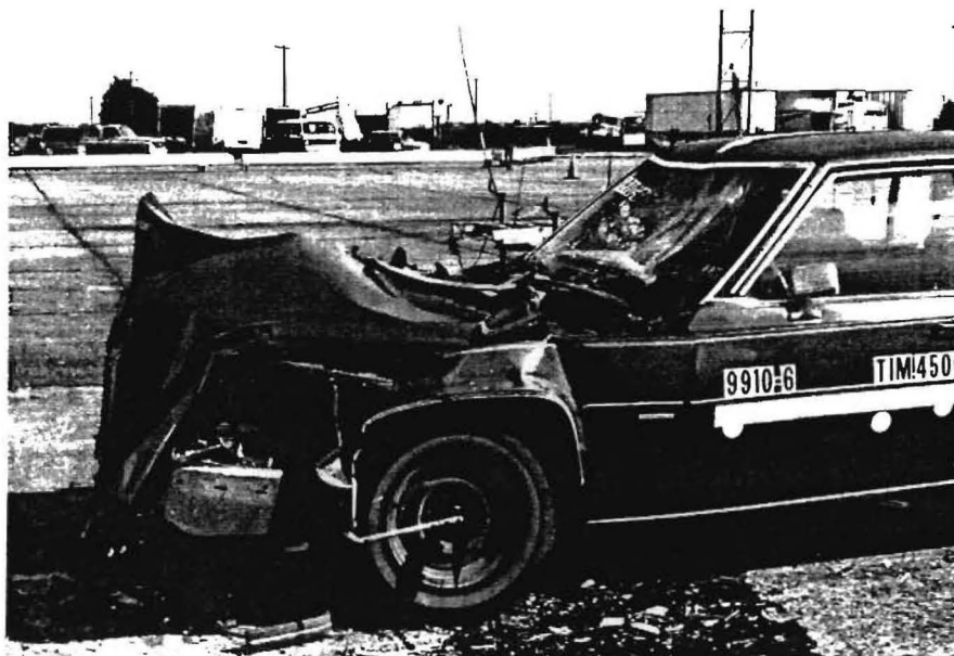
Figure 62 Vehicle after impact with Hecel Model 4000 TMA (9910-6).
