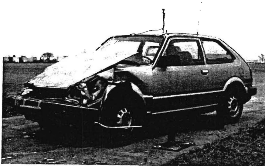
Figure 131. Vehicle after impact with Energy Absorption Hex-foam TMA (9910-8).
